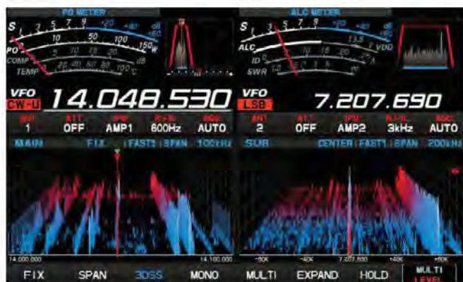
Figure 6 — Same as Figure 5, except a second spectrum view of the sub-receiver display has been added to the right of the first. Note that the second is on a different band, bandwidth, mode, and antenna. Either can be anywhere within the FTdx101MP's tuning range. The two displays can also be one above the other, if you prefer — lots of flexibility available.
