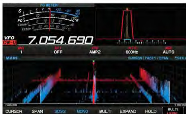
Figure 5 — Same as Figure 4, except we have tapped the 3DSS on-screen button, and now have a 3D view with time marching out the back of the screen, instead of the waterfall. This way, you can see what happened before, as well as what's happening now.
