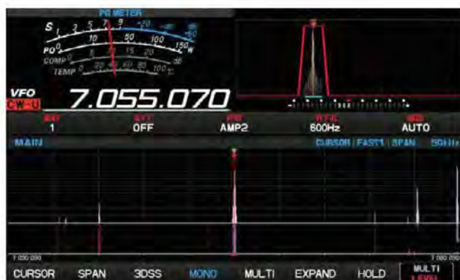
Figure 4 — Screenshot of the Yaesu FTdx101MP display, showing a single panadapter display, with panadapter below, including the frequency tuned by VFO A. The upper right display shows the received bandwidth with the received signal within. The spectrum span can be adjusted from a width of 1 kHz to 1,000 kHz (50 kHz shown) in 10 steps.
