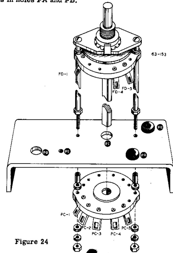
ing holes at FN and FJ. Use lockwashers under the nuts. Now place a 3/8" nut on the switch bushing and secure.
