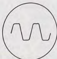
OVERLOADED STAGE, CAUSED BY TOO MUCH SIGNAL INPUT TM4000-52
