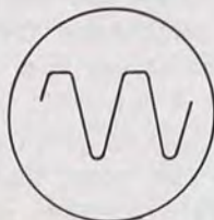
TOO LOW BIAS OR TOO HIGH PLATE OR SCREEN VOLTAGE
