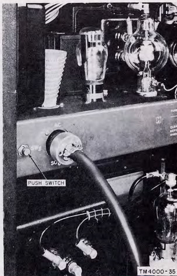
Figure 6. Example of a push-switch interlock.
