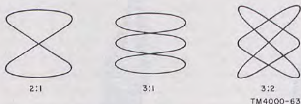
Figure 32. Lissajous figures showing some common frequency ratios.
