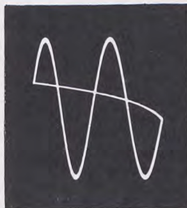
Figure 28. Oscilloscope pattern showing two cycles of a sine wave.
