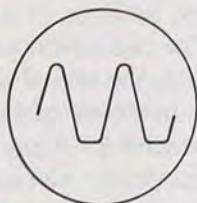
TOO HIGH BIAS OR TOO LOW PLATE OR SCREEN VOLTAGE
