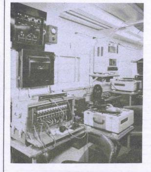
MOBILE RADIO INTERCEPT CENTRAL TRAILER Showing Switchboard BD-72 . View of Interior and Power Control Boxes
