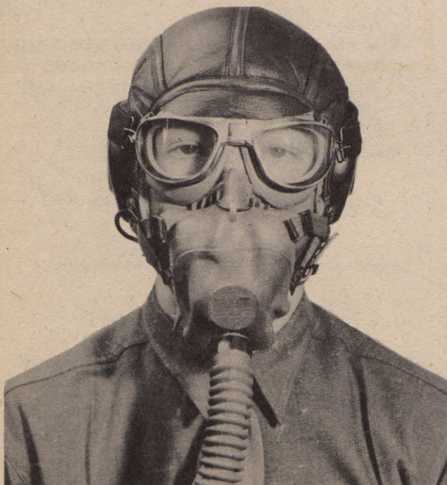
The A-10 Revised demand oxygen mask. Fit is important in all demand masks. Let your Oxygen Officer check the fit.
