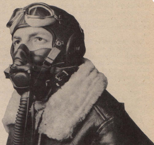
The A-14 demand oxygen mask is the latest type of demand mask available.
