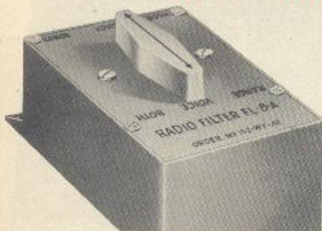
The Radio Range Filter System is designed to separate the 1020-cycle range signal from voice transmissions.
