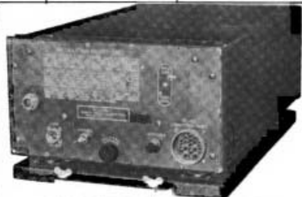
RADIO COMPASS UNIT NR-3/ARN-7 PART OF DEVELOPMENTAL MODEL OF RADIO COMPASS AN/ARN-7
