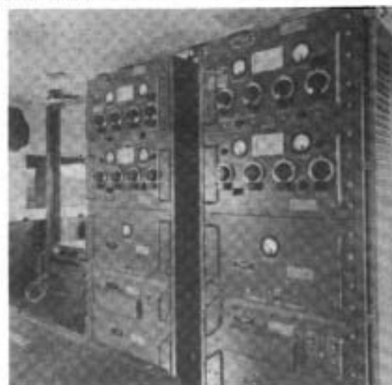
RADIO SET SCR-575, INTERIOR VIEW SHOWING RADIO TRANSMITTERS BC-610 AND CONTROL UNIT RW-27.
