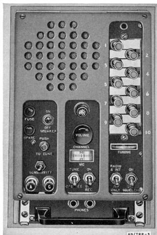
Figure 30. Radio Receiver BC-403, component of Radio AN/TRR-3.
