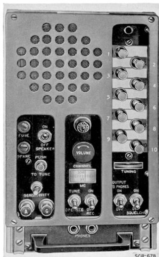
Figure 110. Radio Receiver BC 683-A (front view), component of Radio Set SCR-678.
