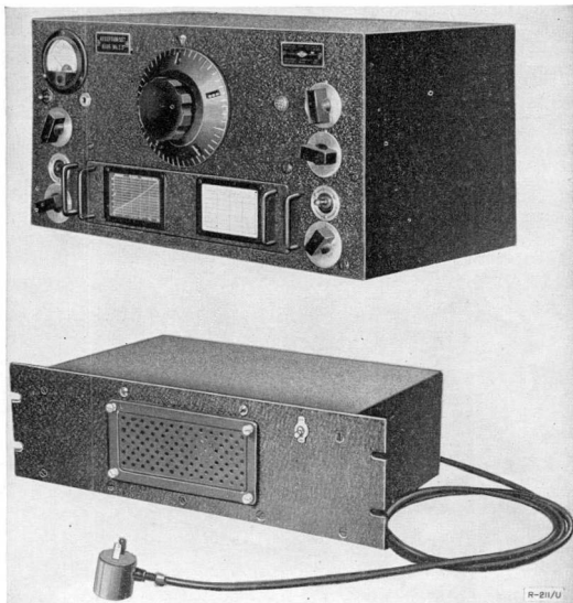
Figure 74. Radio Receiver R-211/U with power supply (National Type SPU-697).
