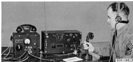
Figure 85. Radio Set SCR-188-A showing components in operating position.
