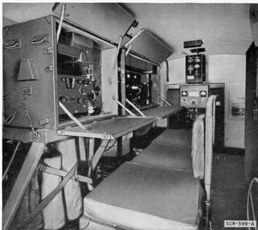
Figure 92. Radio Set SCR-399-A, components installed in Shelter HO-17-A, showing operating positions.
