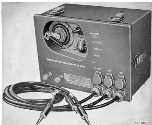
Figure 30. Control Unit RM-39, main component of Remote Control Equipment RC-289.
