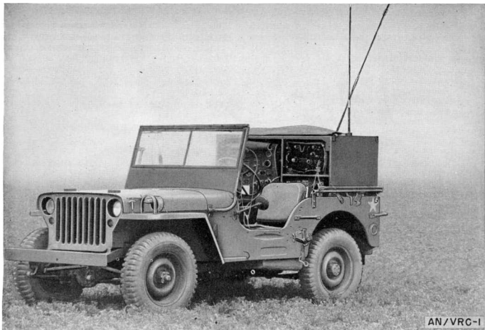
Figure 31. Radio Set AN/VRC-1, prepared for mobile operation.
