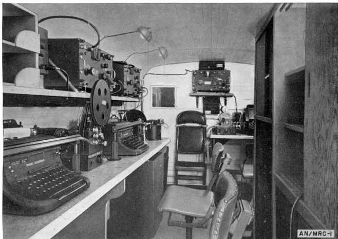
Figure 11. Radio Set AN/MRC-1, components installed in shelter.
