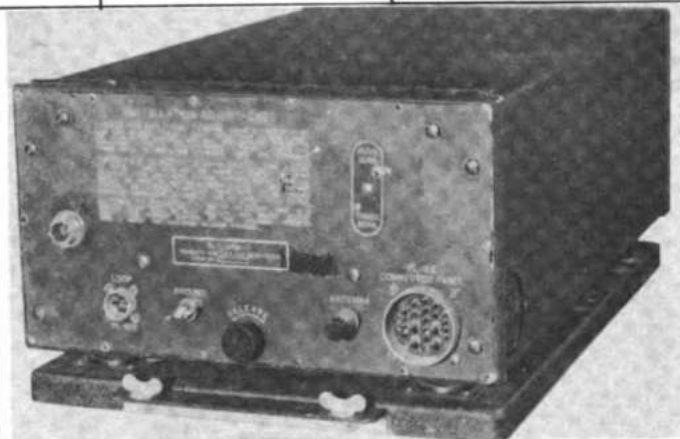
RADIO COMPASS UNIT #R-5/ARN-7 PART OF DEVELOPMENTAL MODEL OF RADIO COMPASS #AN/ARN-7
