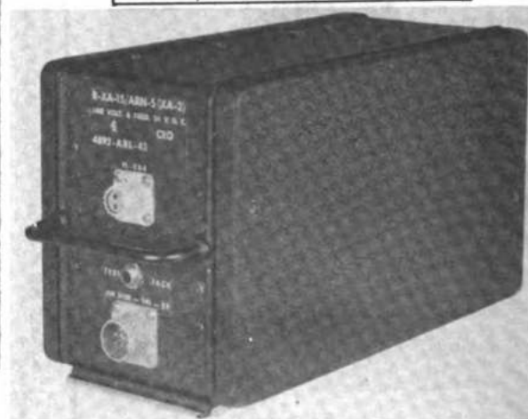
RADIO RECEIVER R-15/ARN-5. PART OF RADIO SET AN/ARN-5. DEVELOPMENTAL MODEL.
