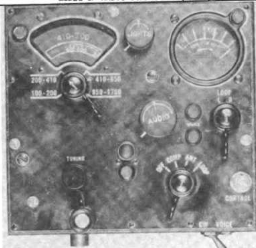
FRONT PANEL VIEW OF RADIO CONTROL BOX #C-4/ARN-7 PART OF DEVELOPMENTAL MODEL OF RADIO COMPASS #AN/ARN-7
