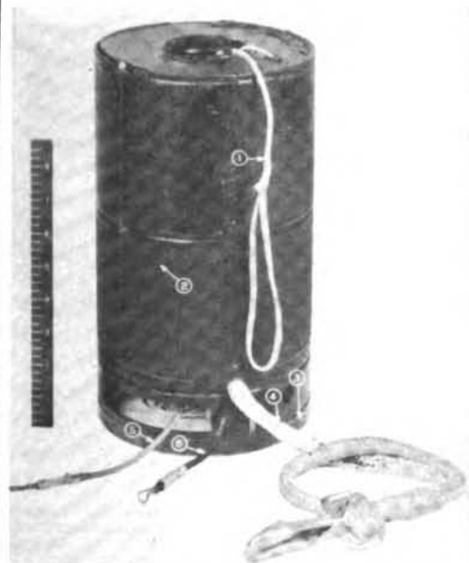
PARACHUTE MX-91/CRN-1; PART OF RADIO TRANSMITTING EQUIPMENT AN/CRN-1
