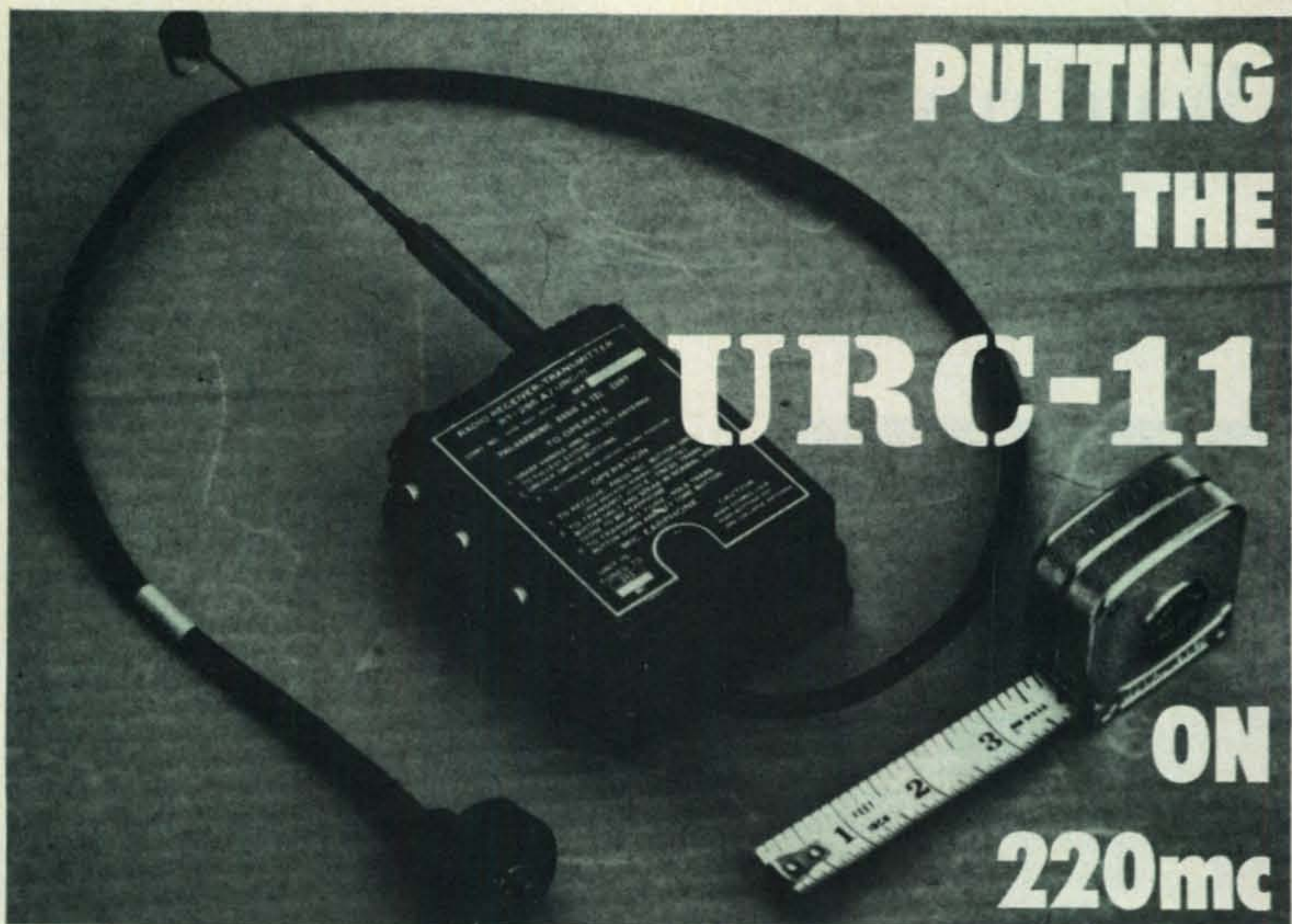
View of the URC-11 Walkie-Talkie showing attached power cable, and antenna partially extended. Scale illustrates very clearly the small size of this unit. (Photo Courtesy W3AY.)
