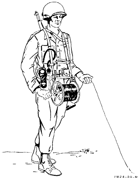
Figure 8-9. Recovering wire with Reel Equipment CE-11 (RL-39 reeling machine with a TA-1 telephone).
