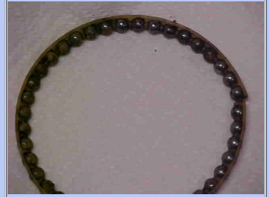
One of the old races with rusty ball bearings and dry grease
