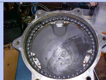
Top bell with upper bearing race (old race with dried grease)
