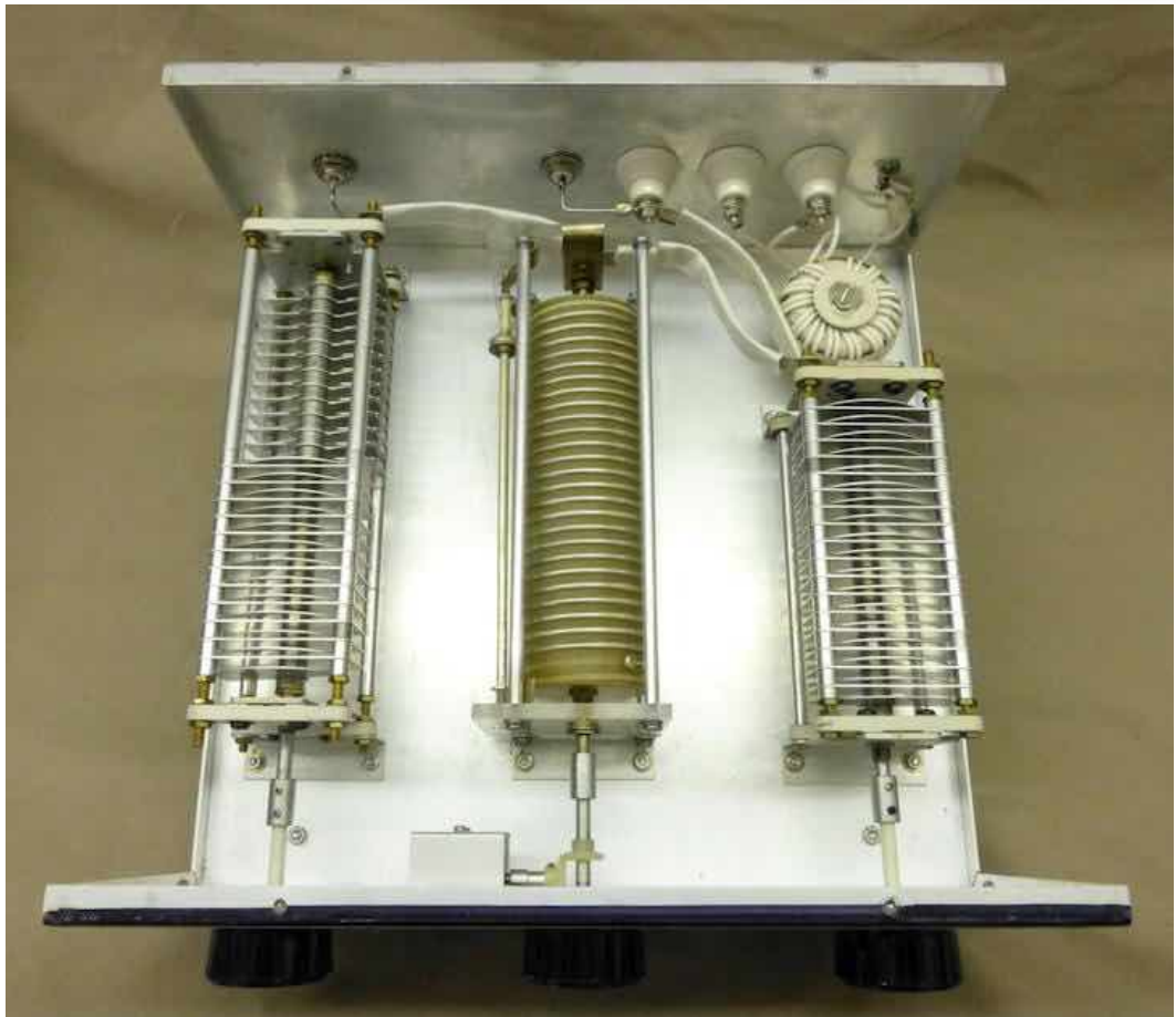
Figure 12: Interior view of the SA-2040. C1 is on the left, and C2 is on the right. Behind C2 is the balun T1. The Inductor L1 is in the center. Photo by Bob Koller - KG7EMO; used with permission.
