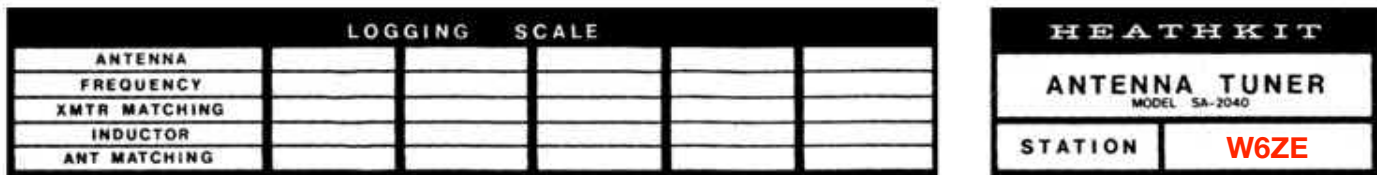
Figure 2: On the front panel is an erasable place to write settings as well as a place to add your station call letters.
