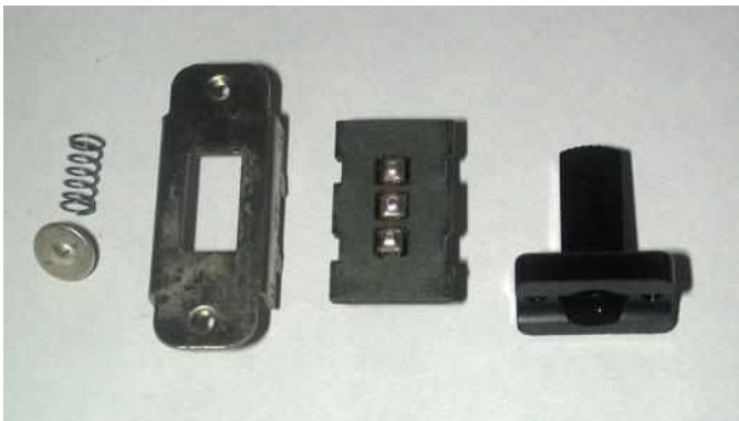
Figure 6: Cleaned Parts: Ready for lubrication and assembly.
