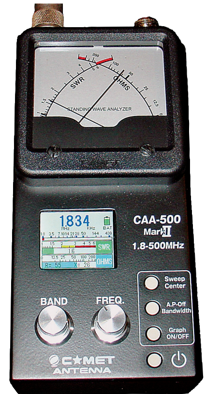
Figure 2 — Fixed frequency measurement of a 160 meter antenna.
