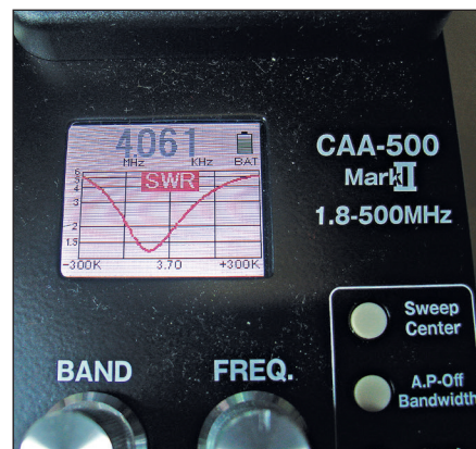
Figure 3 — Swept response measurement of an 80 meter vertical.
