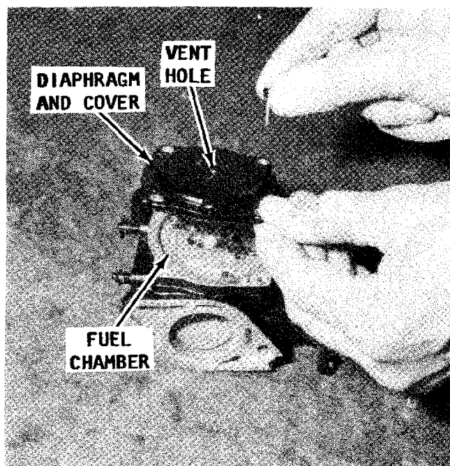
The vent hole for the fuel chamber above the diaphragm must be kept clear to the atmosphere at all times for the diaphragm to function efficiently.
