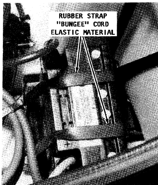
On a Personal Watercraft, two heavy-duty elastic rubber straps, or "bungee" type cords do an excellent job of holding the battery in place, during violent maneuvers.
