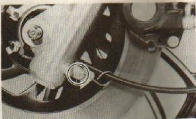
4. Loosen the pinch bolt securing the axle.
