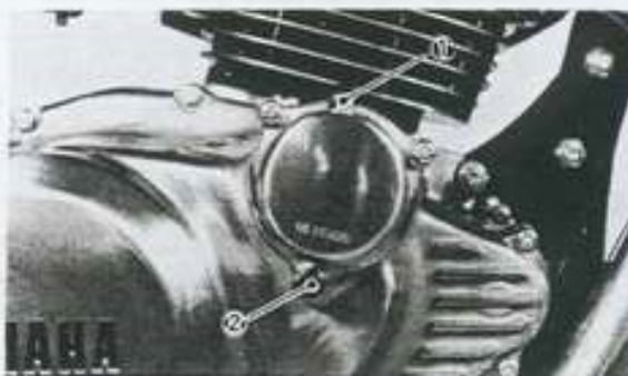
1. Air bleed screw 2. Filter cover screw
