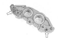
· Tighten each bolt to the specified torque.
