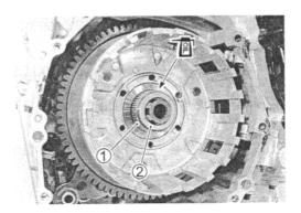
• Install the thrust washer 1.
