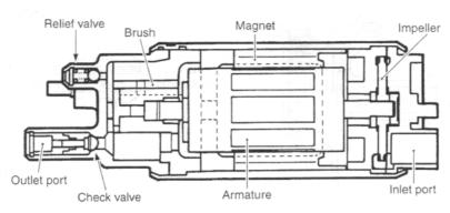
When the impeller is driven by the motor, pressure differential occurs between the front part and the rear part of the blade groove as viewed in angular direction due to fluid friction. This process continuously takes place causing fuel pressure to be built up. The pressurized fuel is then let out from the pump chamber and discharged through the motor section and the check valve.
