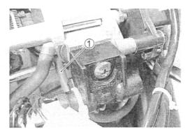
To synchronize throttle valves, remove the respective vacuum hoses ② from each vacuum nipple and connect the vacuum balancer gauge hoses to the vacuum nipples respectively.
