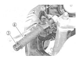
· Remove the handlebar set bolts.
