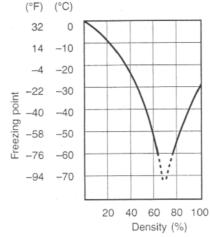
Fig.1 Engine coolant density-freezing point curve.
