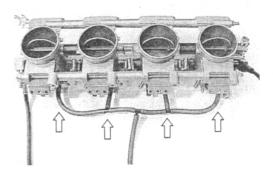
• Remove the TP sensor ④ with the special tool.
