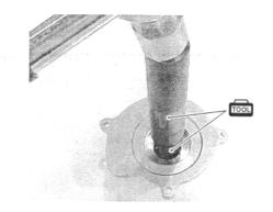
· Apply a small quantity of the SUZUKI SUPER GREASE "A" to the oil seal lip.
