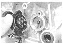
• Apply the THREAD LOCK to the gear position switch bolt, install the gear position switch as shown.
