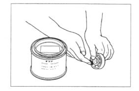
• Install the new bearing to the sprocket mounting drum using the special tool.
