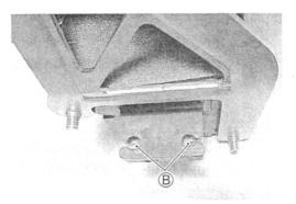
• Turn out the No.1 cable adjuster ② to obtain a cable slack © of 0-1.0 mm (0-0.04 in).
