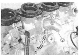
Remove the cylinder head side bolt 4 and its gasket.
