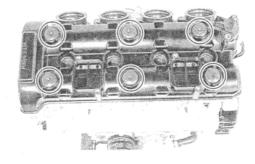
· Remove the dowel pins and O-rings.
