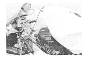
· Remove the air cleaner element by removing the screws.
