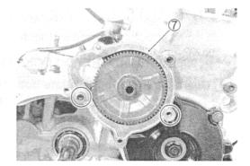
• Install the starter idle gear cover and tighten its bolts to the specified torque.
