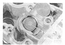
Using special tools, compress the valve springs and remove the two cotter halves ③ from valve stem.
