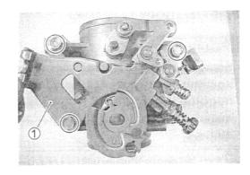
· Install the fast idle link levers properly.
