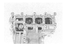
• Tighten the other crankcase bolts a little at a time to equalize the pressure.
