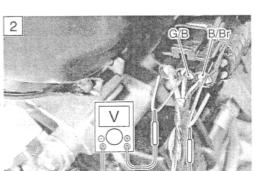
2 Connect the IAP sensor coupler. Insert the copper wires to the lead wire coupler.
