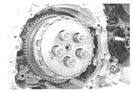
· Hold the clutch housing using the special tool.
