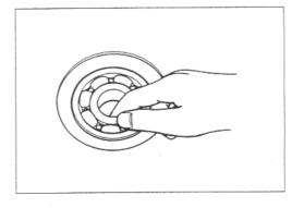
• Remove the wheel bearings by using the special tool (A) or (B).
