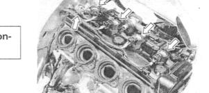
· Remove the ignition coils/plug caps.
