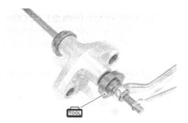
• Apply grease to the bearings, spacers, washers and dust seals.
