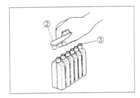
Insert the nozzles of the electrolyte container into the battery's electrolyte filler holes, holding the container firmly so that it does not fall. Take precaution not to allow any of the fluid to spill.
