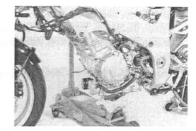
• Remove the engine mounting bolts ①, ②.
