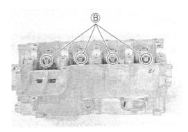
· Apply molybdenum oil solution to the crank pin bearings sur-
