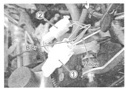
To set the ST valve to fully close position, apply 12 volts to
