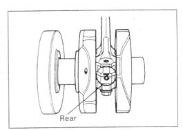
Remove the bearing caps and measure the width of the compressed plastigauge using the envelope scale. This measurement should be taken at the widest part of the compressed plastigauge.
