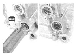
• Install the gearshift cam with the bearing.
