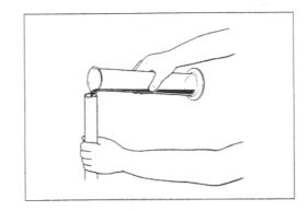
• Move the inner rod slowly with the special tool more than ten times until no more bubbles come out from the oil.
