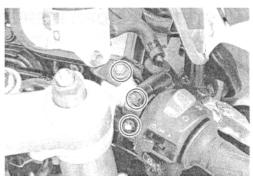
• Remove the reservoir cap ①, insulator ② and diaphragm ③.
