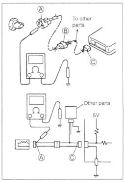
If continuity is indicated, the circuit is shorted to the ground between terminals (A) and (B).
