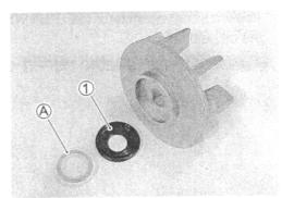
Install the seal washer and the washer onto the impeller securing bolt ②.
