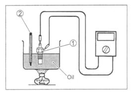
• If the temperature sensor ohmic value does not change in the proportion indicated, replace it with a new one.
