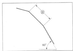
If the contact area W is too low or too narrow, use the 45° cutter to raise and widen the contact area.
