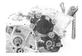
• Remove the shaft ①, wave washer ② washer ③ starter idle gear No.1 ④, bearing ⑤ and washer ⑥.
