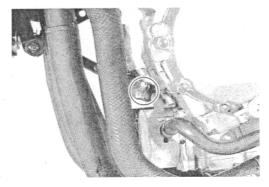
• Disconnect the cooling fan thermo-switch coupler ① and cooling fan coupler ②.
