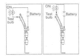
When the switch is immersed in water under the above condition, the bulb should go out. If the bulb remains lit, replace the unit with a new one.
