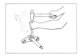
· Drive out the steering stem bearing outer races, upper and lower, using a suitable wedge bar.
