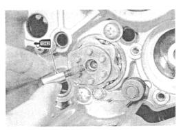
• Install the gearshift shaft/gearshift arm ① with the washers as shown.
