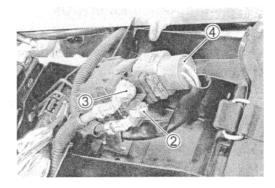
Apply 12 volts to A and B terminals, inspect the continuity between the terminals, positive and negative.
