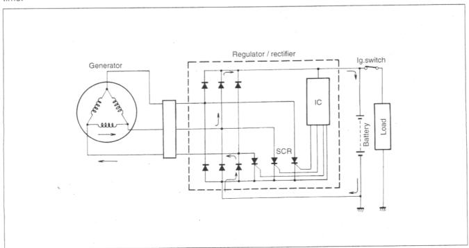
When the engine r/min becomes higher, the generated voltage of the generator also becomes higher and the voltage between the battery terminals becomes high accordingly. When it reaches the adjusted voltage of the I.C., (Integrated Circuit) and it is turned "ON", a signal will be sent to the SCR (Thyristor) gate probe and the SCR will be turned "ON".
