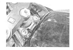
• Lift and support the fuel tank with the fuel tank prop stay 1.
