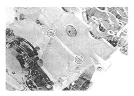
$\bullet\,$  Fit the gasket  $\ensuremath{\textcircled{1}}$  and tighten the water temp. gauge.
