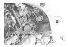
Remove the clutch push rod ①.
