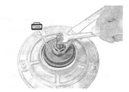
• First install the right wheel bearing, then install the left wheel bearing using the special tool.
