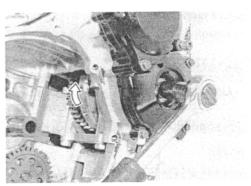
• Install the primary driven gear assembly.
