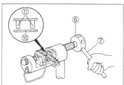
• Continue pressing the joint plate until the distance between the two joint plates come to the specification.
