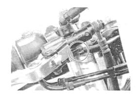
Place a rag underneath the union bolt on the master cylinder to catch any spilt brake fluid. Remove the union bolt and disconnect the brake hose.
