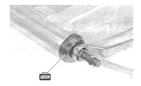
Press the swingarm cushion rod upper side bearing with the special tool.
