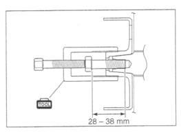
• Remove the generator rotor with the special tool.
