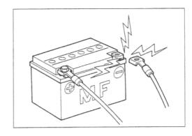
Before measuring voltage at each terminal, check to make sure that battery voltage is 11V or higher. Terminal voltage check at low battery voltage will lead to erroneous diagnosis.
