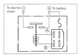
• Check the coil for "open", "ground" and ohmic resistance. The coil is in good condition if the resistance is as follows.
