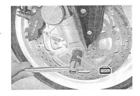
• Tighten the front axle to the specified torque.
