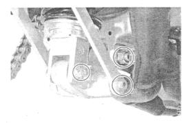
Remove the swingarm pivot shaft lock nut by using the special tool.
