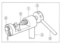
• Stake the joint pin by turning (approximately 7/8 turn) the pressure bolt "A" ③ with the bar until the pin end diameter becomes the specified dimension.
