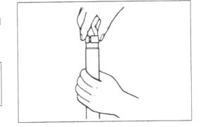
• Apply grease to the oil seal lip lightly before installing it.
