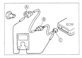
• Disconnect the coupler ® and measure resistance between couplers ® and ®.
