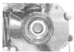
$\bullet$  Remove the cam chain tension adjuster cap bolt  $\textcircled{\scriptsize 1}.$
