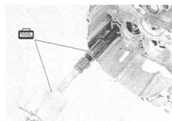
· Remove the gearshift cam bearing using the special tools.
