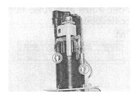
• Remove the fuel pump assy from the fuel pump plate.
