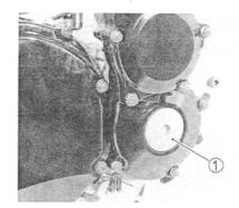
• Turn the crankshaft to bring the line (A) on the starter clutch to the index mark (B) of the valve timing inspection hole and also to bring the cams to the position as shown.
