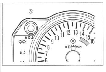
Pointer will return to the starting point right after the completion of the operation. In the case of the pointer not returning to the proper position after doing above, replace the combination meter unit.
