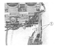
• Loosen the lock nuts 2.
