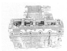
• Remove the crankcase bolts (8 mm).
