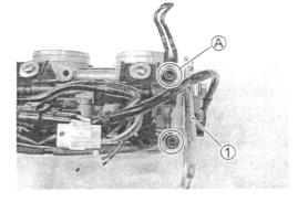
Install the STV actuator to the bracket.
