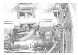
• Connect the proper rubber cap 4 to the nipple on the No.4 throttle body.
