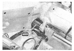
Tighten all engine mounting bolts and nuts to the specified torque. ( 3-12)
