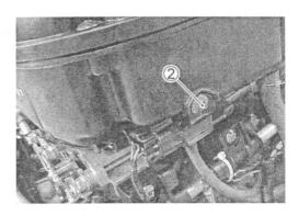
• Diconnect the PAIR vacuum hose 3 from the No. 4 throttle body.
