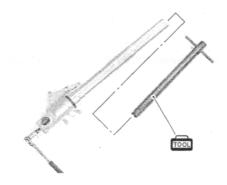
• Remove the inner rod/damper rod (cartridge) 1 and plate 2.
