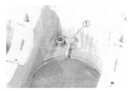
• Remove the oil jet (for transmission) from the lower crankcase.
