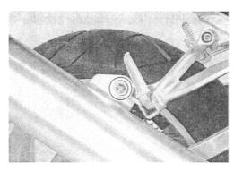
• Remove the radiator mounting bracket 1.
