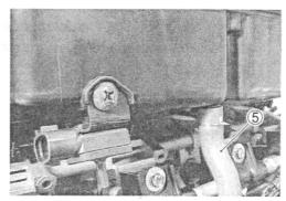
· Loosen the throttle body clamp screws.
