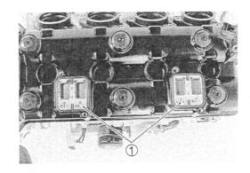
• Apply THREAD LOCK to the bolts, install the PAIR valve and hose. ( 8-22)
