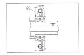
Install the oil pump drive gear 1 to the primary driven gear assembly.
