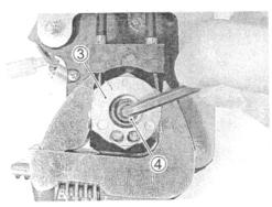
Remove the pulley 3 together with the cables.
