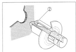
Push in the head of center piece until it becomes flush with the fastener outside face.
