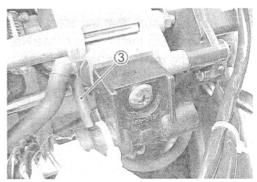
• Connect a proper rubber cap 4 to the nipple on the No. 4 throttle body.
