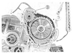
• Install the new gasket 1 and the dowel pins.
