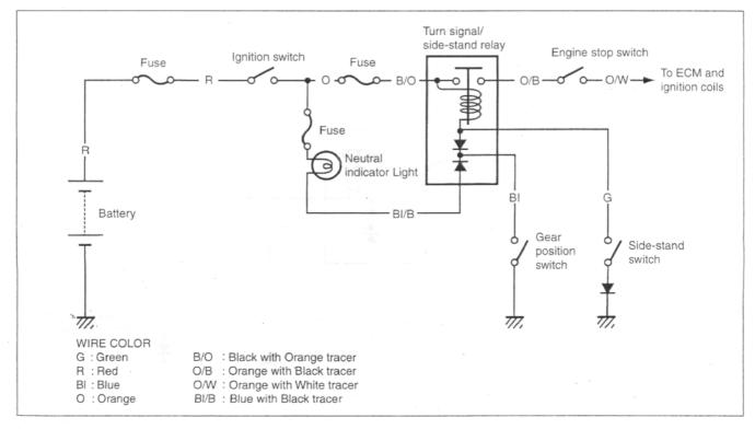
The circuit consists of the turn signal/side-stand relay, neutral indicator light, gear position switch and side-stand switch. The ignition coils will send voltage to the spark plugs dependant on what gear the transmission is in and whether the side-stand is either up or down. The gear position and side-stand switches work together in this system. The ignition coils work only in two situations as follows.
