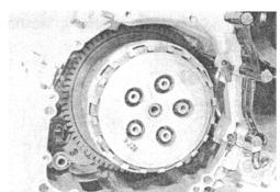
• Remove the clutch push piece ①, the bearing ② and the thrust washer ③.
