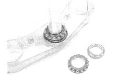
· Remove the steering stem lower bearing inner race with a chisel.
