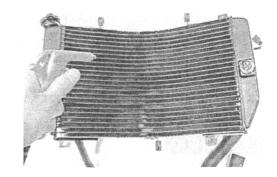
Fins bent down or dented can be repaired by straightening them with the blade of a small screwdriver.
