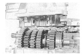
Tighten the crankcase bolts a little at a time to equalize the pressure.
