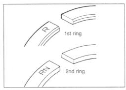
Position the gaps of the three rings as shown. Before inserting each piston into the cylinder, check that the gaps are so located.
