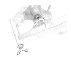
• Draw out the swingarm pivot bearings ① and the swingarm cushion rod upper bearings ② with the special tools.
