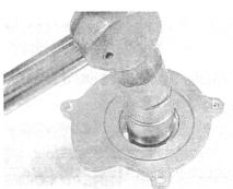
· Install the new bearing using the special tool.
