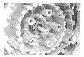
· Unlock the clutch sleeve hub nut.
