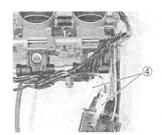
Install the throttle body to the engine and connect the injector lead wire coupler ⑤.
