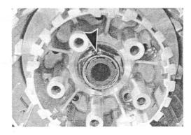
• Insert the clutch drive plates and driven plates one by one into the clutch sleeve hub in the prescribed order.
