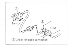
• Using a test male terminal, check the female terminals of the circuit being checked for contact tension.
