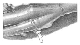
• Drain engine coolant. ( 2-18)
