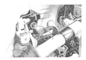
• Apply the grease to the throttle cables and their holder.
