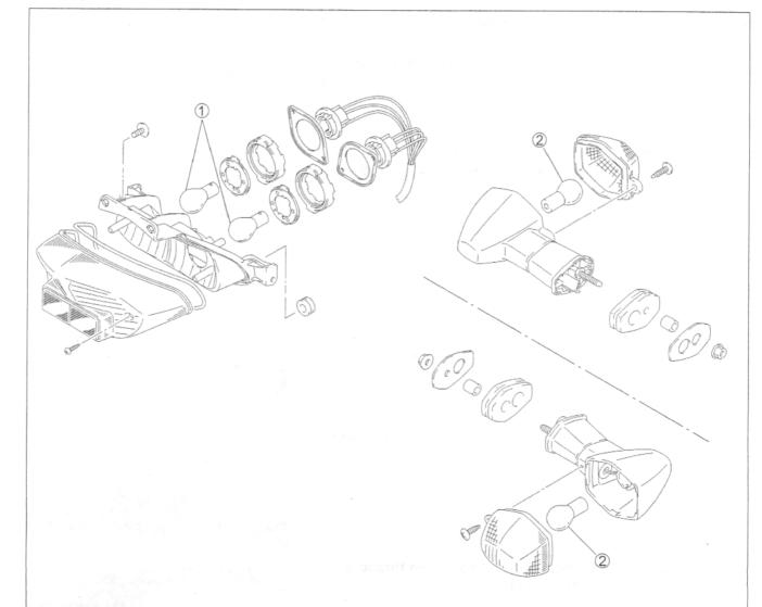
Brake light / Taillight bulb ①: 12V 21/5W  $\times$  2 Turn signal light bulb ②: 12V 21W  $\times$  4
