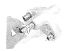
· Draw out the cushion lever bearings with the special tool.
