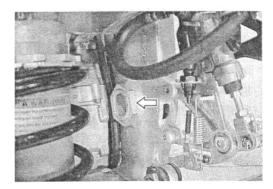
· Remove the swingarm pivot boss by removing its set screws.
