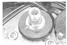
• Tighten the steering stem lock nut to the specified torque with the special tools.
