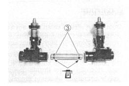
• Assemble the fuel delivery pipes as show in the illustration.
