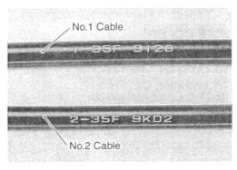
\* No.2 inner cable is longer than that of No.1 cable.
