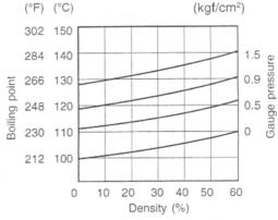
Fig.2 Engine coolant density-boiling point curve.
