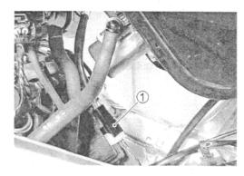
· Place a rag under the fuel tank and disconnect the fuel feed hose 2.
