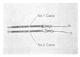
· Connect the two cables temporarily to the throttle body.
