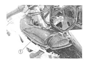
• With the fastener removed, remove the left air intake pipe 2.
