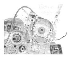
Apply SUZUKI BOND "1207B" light to the groove of the signal generator lead wire gromet.
