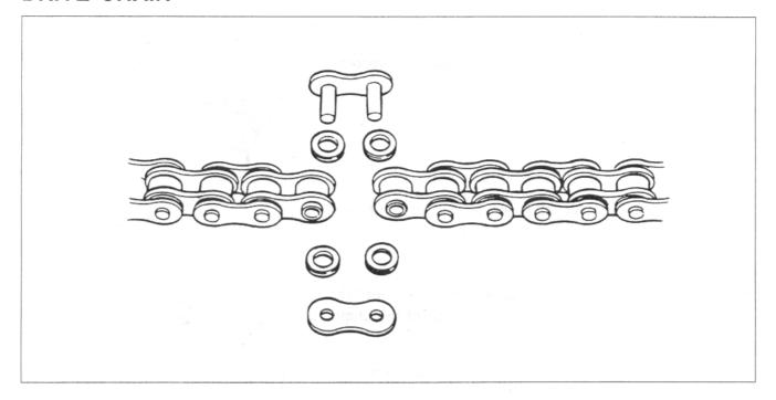
Use the special tool in the following procedures, to cut and rejoin the drive chain.
