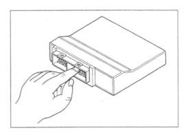
When disconnecting and connecting the ECM couplers, make sure to turn OFF the ignition switch, or electronic parts may get damaged.
