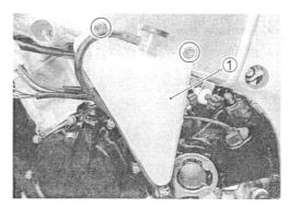
5-12 COOLING AND LUBRICATION SYSTEM • Remove the engine sprocket cover 1. · Disconnect the water hoses. · Remove the water pump. · Remove the water pump cover. · Remove the impeller securing bolt ② by holding the impeller shaft with a water pump pliers.
