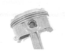
· Apply engine oil to the sliding surface of the pistons and cylinder walls.
