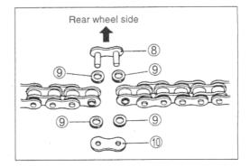
Apply grease on the recessed portion of the joint plate holder
