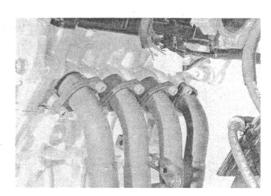
· Remove the muffler mounting bolt and nut.
