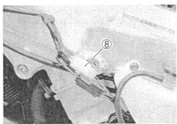
Disconnect the lead wire couplers from each ignition coil/plug cap and camshaft position sensor.
