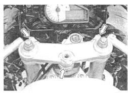
With the handlebar clamp bolts loosened, draw out the handlebars to upward.
