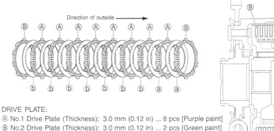
DRIVEN PLATE: (a) No.1 Driven Plate (Thickness): 1.6 mm (0.09 in) ... 2 pcs
