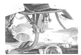
Remove the steering stem lock nut, the washer and the steering stem nut with the special tools.
