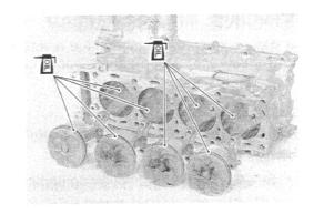
• Install the pistons and conrods into the cylinders from upside.
