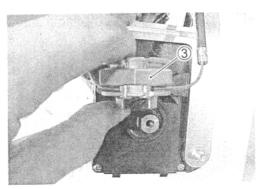
• Disconnect the two cables from the throttle body.
