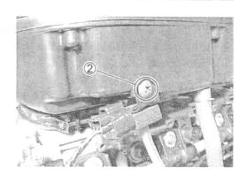
• Disconnect the vacuum hose 3 from the No.4 throttle body.
