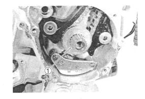
• Install the starter clutch assembly onto the crankshaft.
