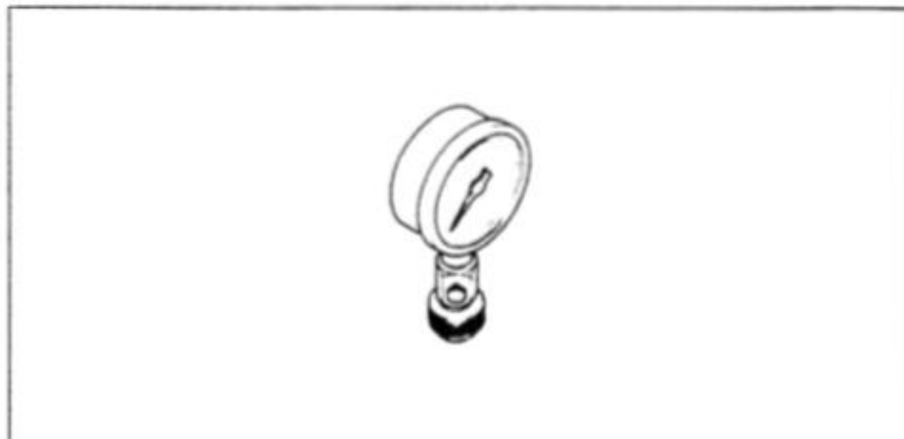
Compression Gauge Adapter, M10 X 1.0: 57001-1317
