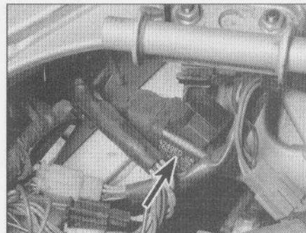
13.3 Location of the turn signal flasher (arrow)
