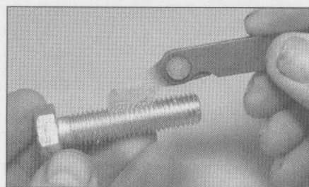
2.12 Using a thread gauge to measure pitch
