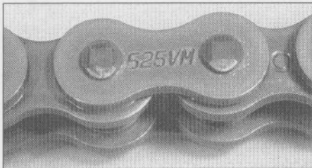
8.10 Typical chain size and type marking
