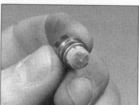
8.3e Clean needle valve seat filter and renew the O-ring
