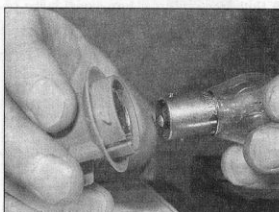
21.5b Note offset pins on bulb to prevent incorrect installation
