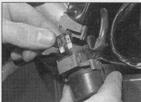
7.1b On ZX1000 B and ZX1100 C/D models main fuse is fitted to starter relay - ZX1100 C shown
