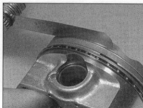
25.4 Checking piston ring to groove clearance
