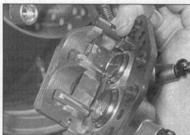
8.11c Ensure pad springs are correctly fitted. Do not omit the piston insulators (where fitted)
