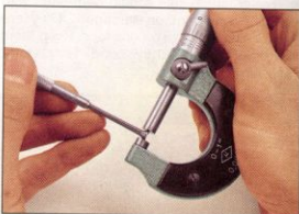
3.10 ... then measure the gauge with a micrometer
