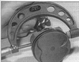
25.3 Measuring piston diameter
