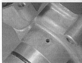
9.1 Examine drainage hole for signs of coolant leakage
