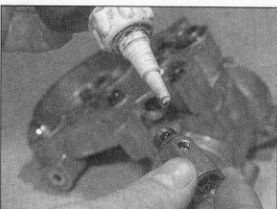
19.3 On refitting apply thread-locking compound to its threads
