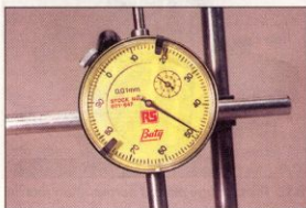
3.17 Dial gauge reading of 1.48 mm
