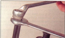
2.18 Two nuts can be locked together to unscrew a stud from a component
