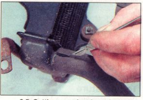
9.5 Cutting a coolant hose free with a sharp knife
