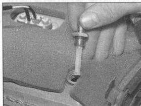
17.2 On ZX1100 C/D models fuel filter is separate from the fuel tap and is a screw fit in the tank
