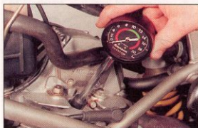
3.20 Using a rubber-cone type cylinder compression gauge
