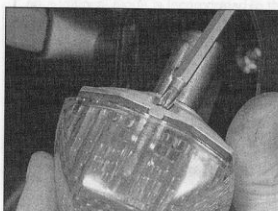
21.6b ... remove lens assembly and slacken two screws which secure lens to the bulbholder
