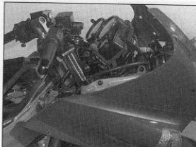
23.17b Offer up the upper fairing section . . .
