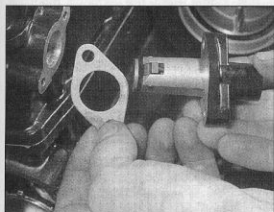
45.9a Fully retract the tensioner pushrod and refit the tensioner using a new gasket
