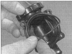
8.13b Fit a new O-ring to thermostat housing cover ...
