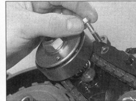
41.2c ... washer and bolt - apply thread-locking compound to the bolt and tighten it securely
