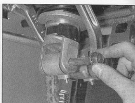
13.9c . . . and the lower suspension unit bolt; tighten all to their specified torque settings
