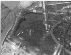
4.1 Spark plugs can be removed using plug spanner supplied in machine's tool kit
