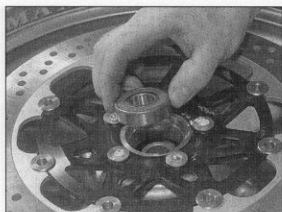
6.5c Grease the cavity and fit the second bearing
