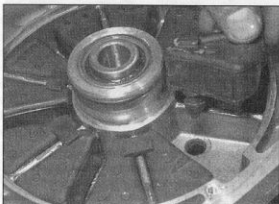
Cush drive rubbers dampen out transmission shocks
