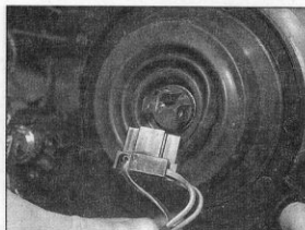
21.3c Ensure rubber bulb cover is correctly installed and refit the headlamp connector
