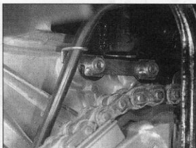
14.3a Note bracket which front two left-hand footrest bracket bolts screw into
