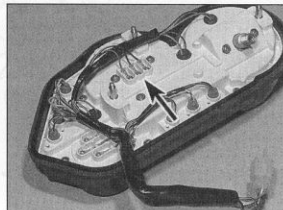
20.4 Disconnect the tachometer wiring connectors (arrowed) before attempting to remove it from the panel
