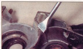
7.3 Paper gaskets can be scraped off with a gasket scraper tool ...
