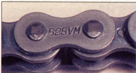
8.10 Typical chain size and type marking
