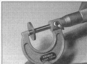
Tappet shims are measured with a micrometer
