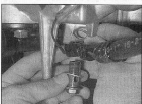
46.9 Fit a new sealing washer on each side of all oil cooler hose unions
