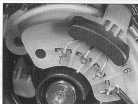
6.6 Unsolder terminal wires quickly to avoid damaging the rectifier
