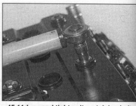
45.11d . . . and tighten its retaining bolts evenly and progressively to the specified torque setting
