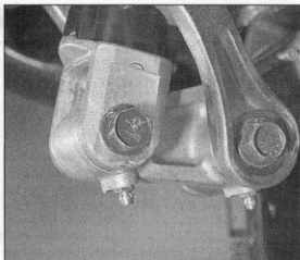
21.1 Where provided, lubricate swinging arm and suspension linkage via the grease nipples
