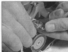
34.2c ... refit the shouldered spacer as shown and tighten its retaining nut securely
