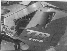
23.17g Offer up the lower fairing sections . . .
