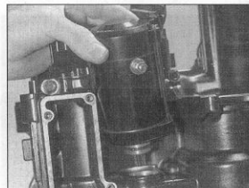
38.3 Apply engine oil to starter motor O-ring and install starter motor, tightening its bolts securely
