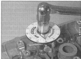
Angle-tightening cylinder head bolts
