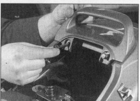
25.2 Grab rail is retained by two bolts
