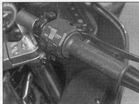
7.1 Throttle cable freeplay is measured in terms of twistgrip rotation
