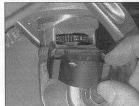
2.17 Remove plastic cover to gain access to rear suspension damping adjuster on ZX1100 C/D models
