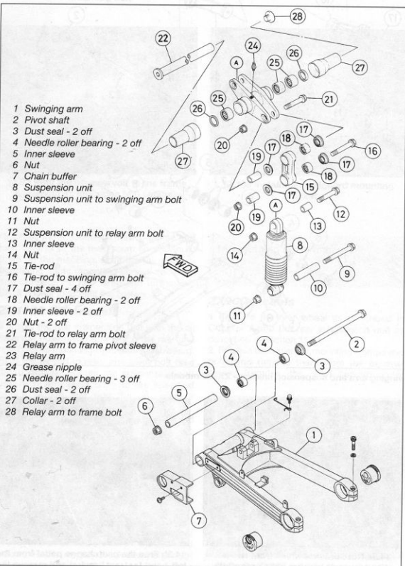
14.5 Swinging arm and suspension linkage - ZX1000 A models
