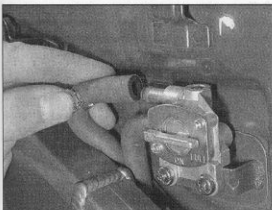
3.3a On ZX1100 C models do not disconnect the lower fuel tap hose
