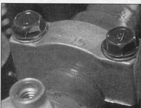
45.5b . . . and install the bearing caps using the arrows and numbers cast into the top surface
