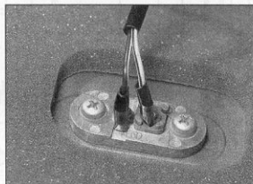
16.8 Fuel level sensor unit is retained by two screws
