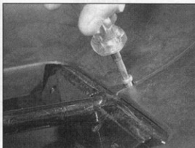
23.4a Slacken the upper inner fairing retaining screws and carefully remove the inner fairing sections
