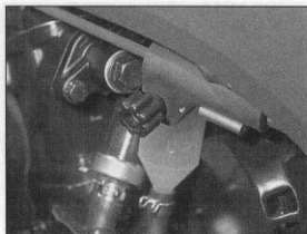
7.9 Idle speed adjuster is situated on left-hand side carburettors - ZX1100 C/D shown
