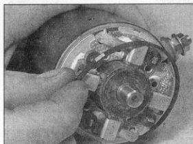
9.11d Fit a new O-ring . . .
