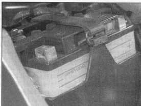
3.2 Electrolyte level must be between marks on casing
