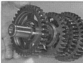
31.12b ... followed by the 3rd gear pinion
