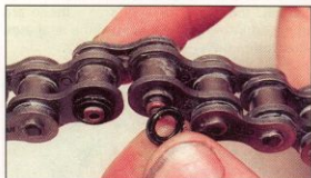
8.5 ... install the O-rings over the pin ends ...
