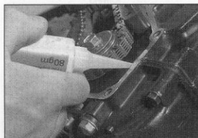
41.4a On ZX1000 B and ZX1100 C/D apply silicone sealant as described in text before fitting new gasket
