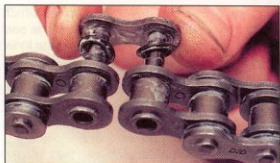
8.4 Insert the new soft link, with O-rings, through the chain ends ...
