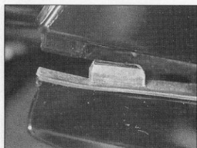
23.7a On refitting do not omit rubber dampers which are fitted to the tangs on the middle fairing section . . .
