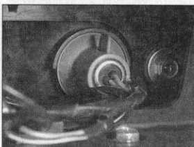
21.5a Stop/tail lamp bulbholders are removed from inside the tail section
