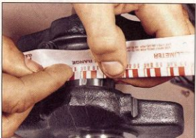
3.16 Measuring the width of the crushed Plastigauge
