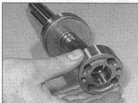
31.7c Fit the clutch drum centre collar with its flat surface facing the thrust washers ...
