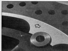
8.3 Where discs show a stamped arrow ensure this faces in normal direction of wheel rotation
