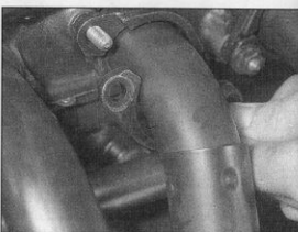
46.5c Refit the exhaust pipe front clamps and nuts and tighten as described in text
