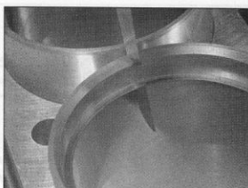
25.5 Measuring piston ring end gap
