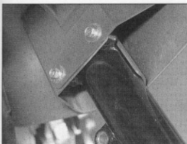
2.2a Mudguard retaining bolts are on the inside of the mudguard
