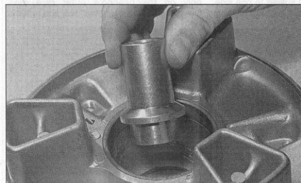
7.4 Do not omit spacer from sprocket carrier on reassembly
