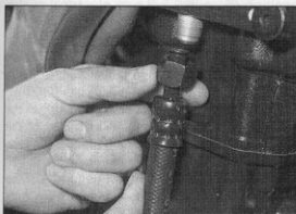
9.4 ZX1000 B and ZX1100 C/D models remove oil hose which runs down right-hand side of cylinder block
