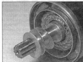
9.12a On ZX1000 and ZX1100 C/D models refit front commutator shims in their original positions . . .
