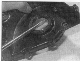
20.4a Carefully lever out old oil seals using a flat-bladed screwdriver ...
