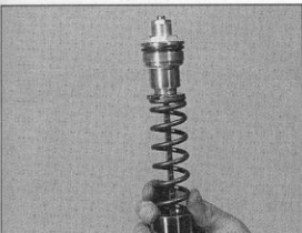
3.10a On ZX1100 C models fit the fork spring, spring seat and top plug as an assembly ...
