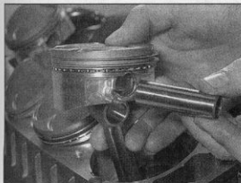
42.2b Insert the gudgeon pin into the piston . . .
