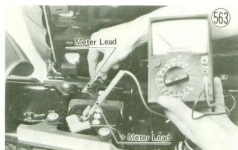
Regulator Test (In Circuit)
