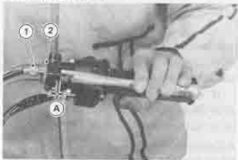
1. Adjuster 2. Knurled Locknut A. 2 ~ 3 mm (0.08 ~ 0.12 in)
