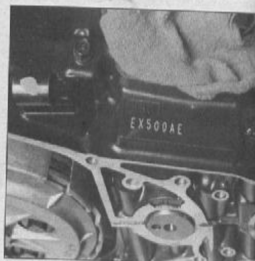
The engine serial number is located on the right side of engine case
