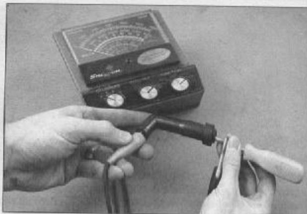
2.5 Unscrew the spark plug caps from the plug wires and measure their resistance with an ohmmeter
