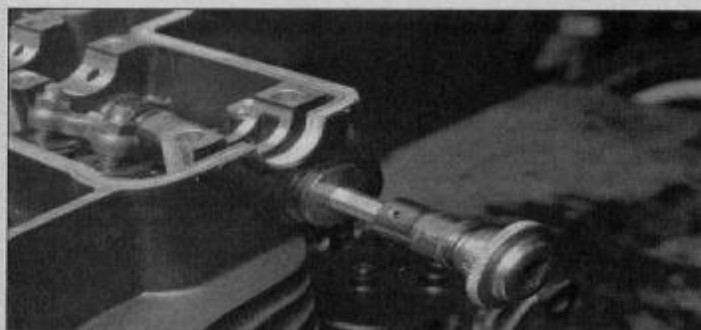
9.30a Insert an Allen wrench into the rocker shaft head (a bit like this one is necessary for tightening the plug to specifications). . .
