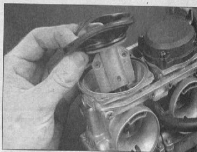
7.4 Remove the diaphragm/piston assembly from the carburetor body
