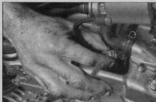
15.2a Rotate the spark plug caps back and forth to loosen them...
