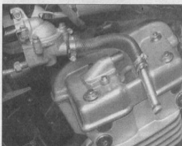
9.3 Pull the tubes out of the cylinder head and remove the O-rings with a pointed tool
