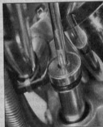
29.2c ... once the retaining ring is removed, release the spring pressure
