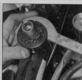
25.8 Use a spanner wrench like this one to loosen or tighten the steering stem locknuts (upper triple clamp removed for clarity)
