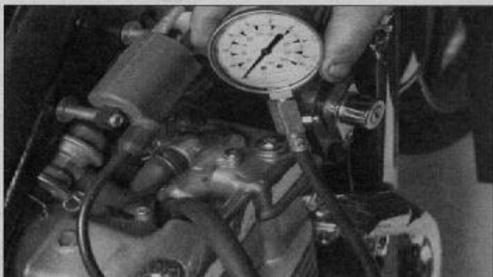
14.5 A compression gauge with a threaded fitting for the spark plug hole is preferred over the type that requires hand pressure to maintain the seal
