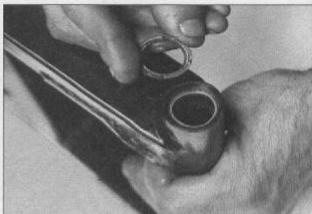
8.8c ... and pry out the grease seals for access to the bearings
