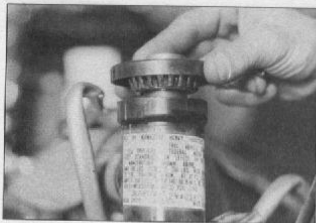
5.9 Lift off the race cover and upper bearing
