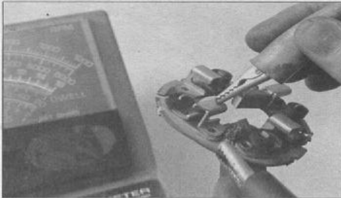
27.10 There should be no continuity between the brush plate and the brush holders (the resistance should be infinite) (EN450 model shown)
