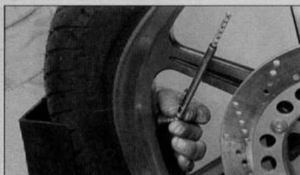
8.4 Use an accurate gauge to check the air pressure in the tires
