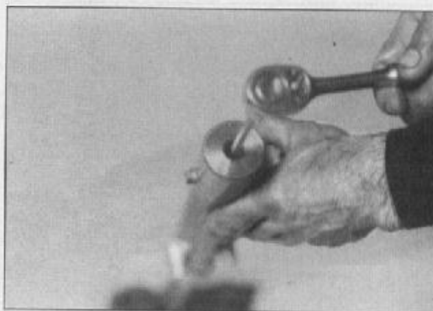
4.4b Hold the damper rod and remove the screw with an Allen wrench
