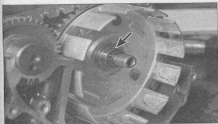
25.2 Slip the clutch housing back-and-forth to expose the inner bearing sleeve (arrow), then pull it out
