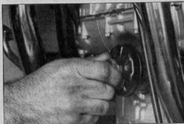
12.5a Remove the oil filter with a filter wrench or a special socket; the special socket is best, since it allows the filter to be tightened accurately with a torque wrench
