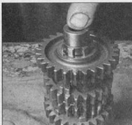
30.11h ...then secure the gear and washer with a snap-ring
