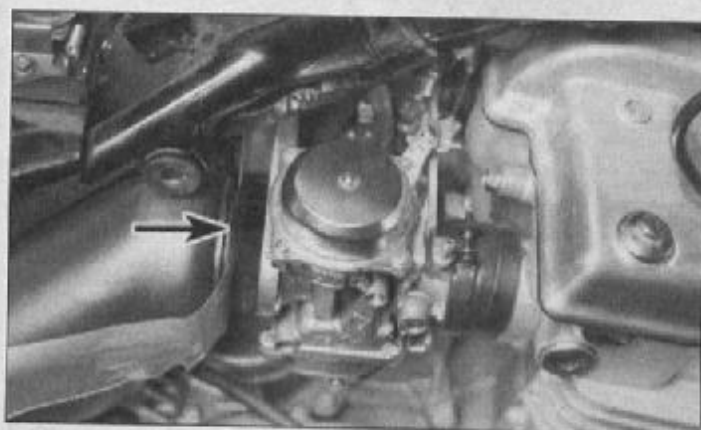
6.6b ... then separate the air inlet ducts from the air box and place a piece of tape (arrow) over the air box openings
