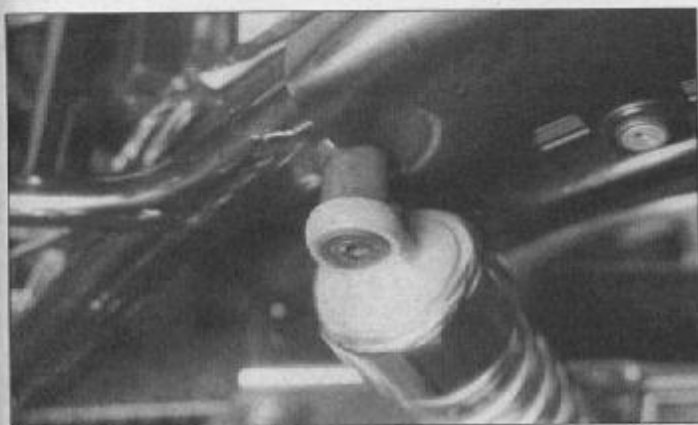
6.3b Once the bolt is removed, the upper end of the shock absorber can be detached from its mounting bracket
