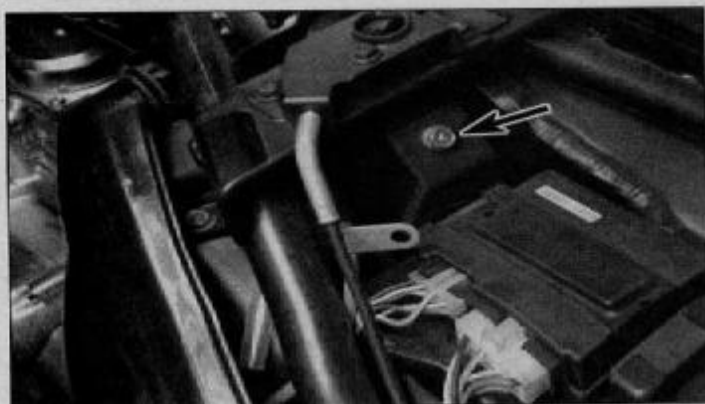
4.3 Remove the junction box bracket bolt (arrow) and lift the junction box to uncover the battery
