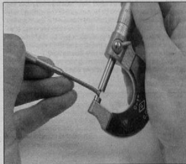
12.16b Measure the small hole gauge with a micrometer
