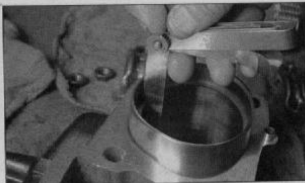
15.3b . . . then check the piston ring end gap with a feeler gauge
