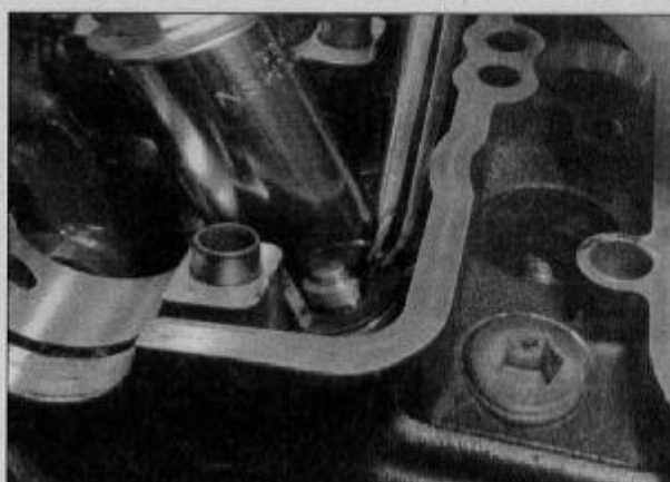
12.7b Remove the valve keepers/collets with needle-nose pliers or tweezers
