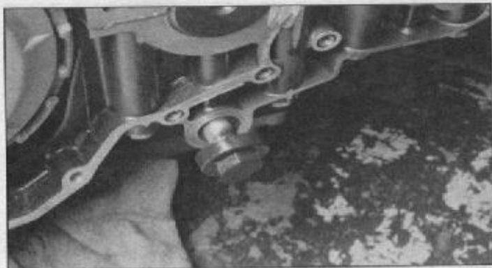
23.2c ...and the oil passage plug so all the lines and passages can be cleaned
