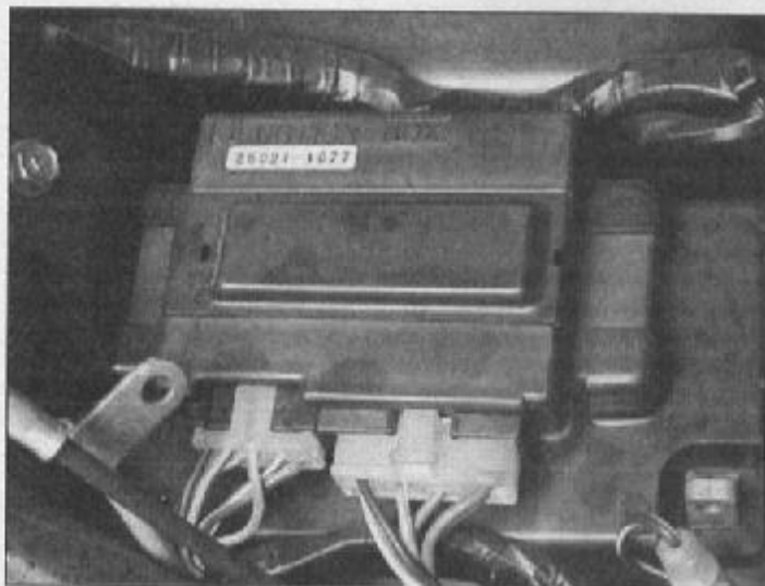
5.2a Most of the EN500 fuses, including the spares, are located on the junction box
