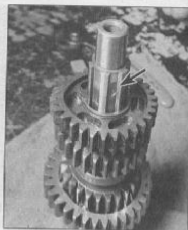
30.17j . . .and secure them with a snap-ring; the slots in the shaft (arrow). . .
