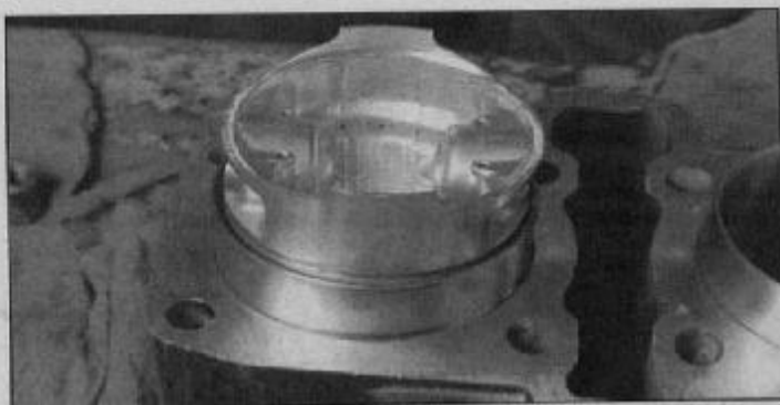
15.3a Square the ring in the bore by turning the piston upside down and tapping on the ring. . .
