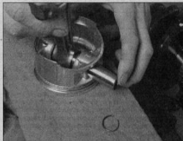
14.15 Slip the pin into the piston and try to wiggle it back-and-forth; if it's loose, replace the piston and pin
