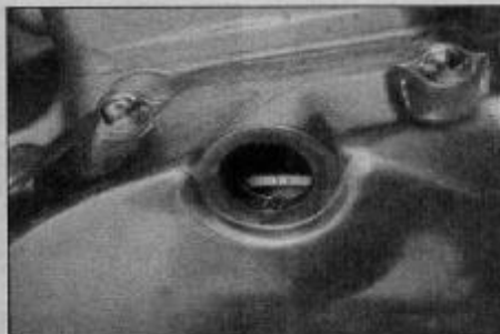
17.6b . . . until the T mark on the rotor aligns with the timing notch . . .
