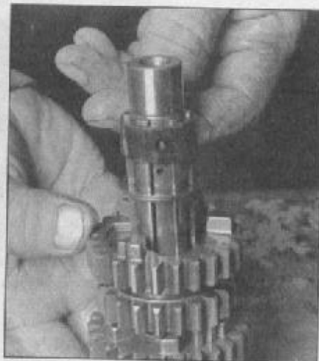
30.11f ...Align the oil hole in the sixth gear bushing with the oil hole in the shaft, then slide the bushing down against the toothed washer
