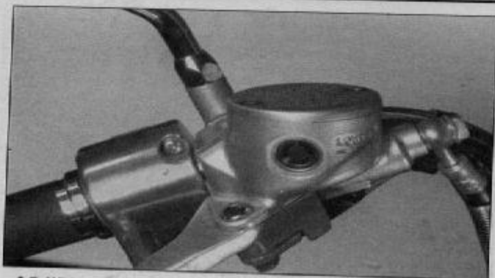
3.7 With the master cylinder in a level position, check the fluid level in the inspection window
