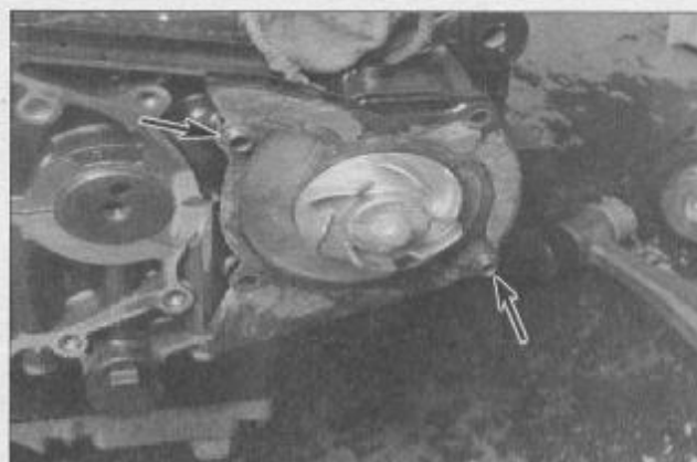
8.18 Position the housing on the engine, install a new gasket and the dowels (arrows); turn the impeller counterclockwise (anticlockwise) to install it on the shaft
