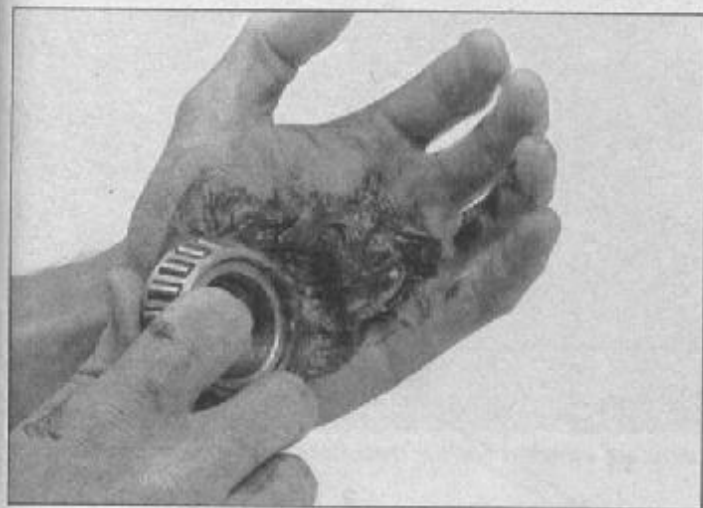
5.19 Work the grease completely into the rollers
