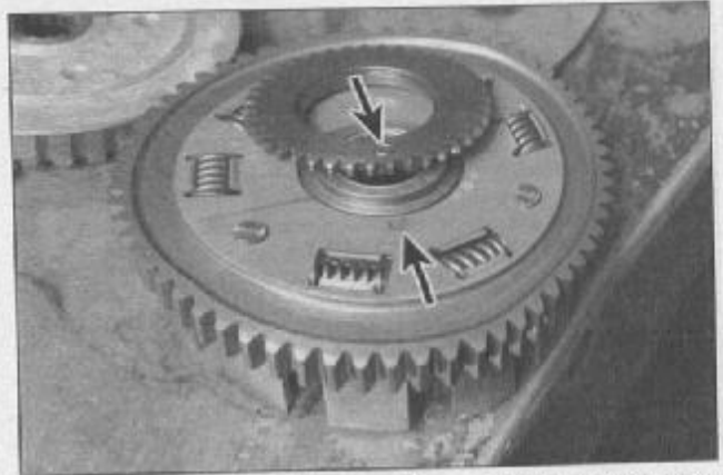
25.30a The pin in the oil pump drive gear must engage the notch in the clutch housing (arrows)...
