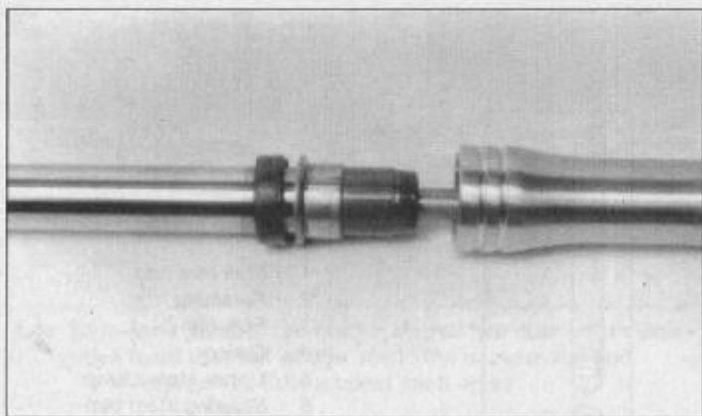
4.17a Install the assembled inner fork tube into the outer fork tube...
