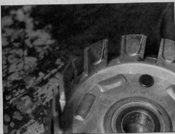
19.15 Check the slots on the clutch housing for indentations - if they're worn, the crankcase will have to be disassembled to remove the clutch housing
