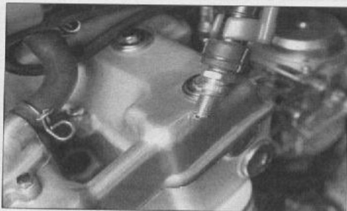
2.3 With the wire attached, ground (earth) a spark plug to the engine and operate the starter - bright blue sparks should be visible
