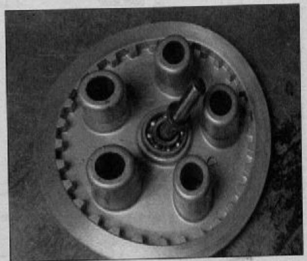
19.16 Check the pushrod and the bearing in the spring plate for wear and damage
