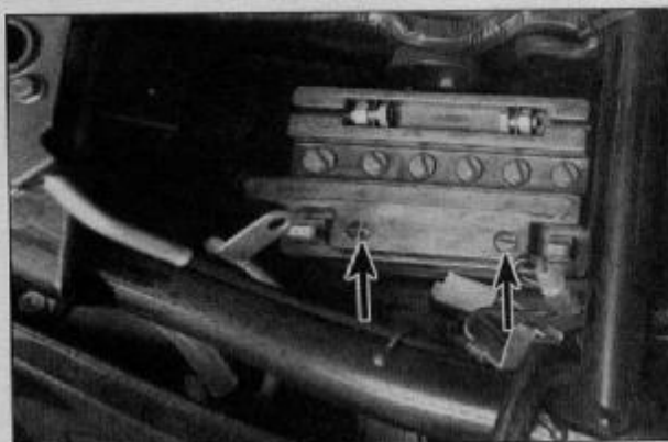
4.4 The positive terminal is identified by a plus mark molded into the top of the battery and the negative terminal is identified by a minus mark (arrows); ALWAYS disconnect the negative cable first and connect it last to prevent sparks which could cause a battery explosion
