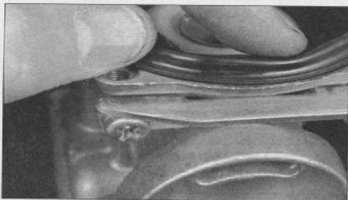
8.8 Make sure the bead of the vacuum diaphragm seats in its groove, and that the diaphragm isn't distorted
