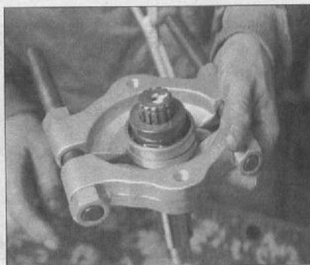
30.15p If the bearing is worn or damaged, place it in a bearing splitter, press it off the shaft and press a new one on (or have the job done by a motorcycle dealer)
