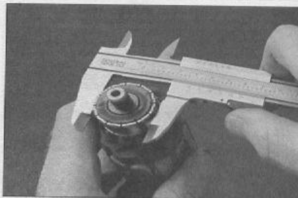
27.7 Check the commutator for cracks and discoloring, then measure the diameter and compare it with the minimum diameter listed in this Chapter's Specifications
