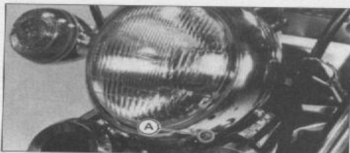
10.5 The vertical adjusting screw on EN500 models is low on the left side of the headlight ring
