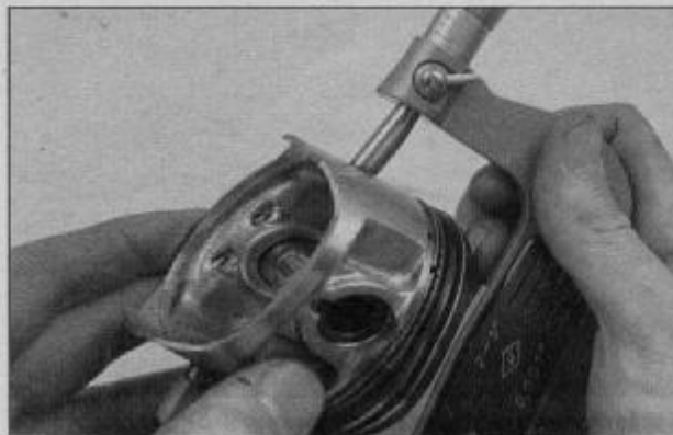
14.14a Measure the piston diameter with a micrometer
