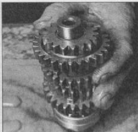
30.11i Install second gear. . .
