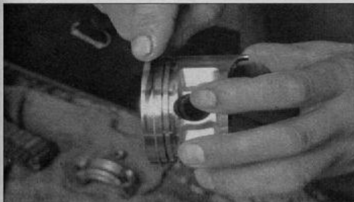
14.13 Measure the piston ring-to-groove clearance with a feeler gauge
