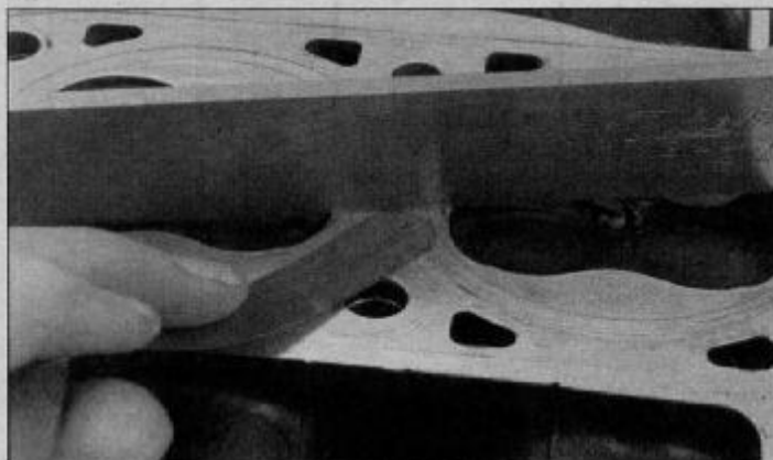
12.14 Lay a precision straightedge across the cylinder head and try to slide a feeler gauge of the specified thickness (equal to the maximum allowable warpage) under it
