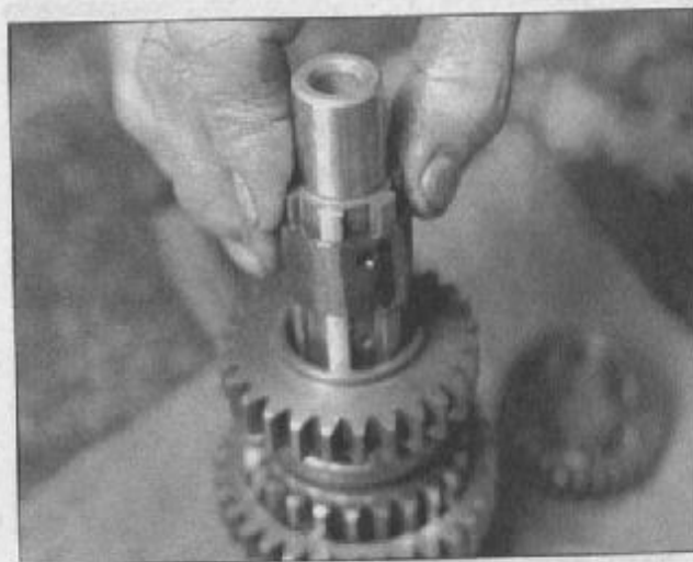
30.17g . . .and its bushing (align BOTH oil holes in the bushing with those in the shaft)
