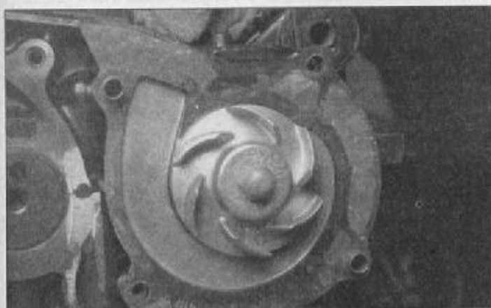
8.5 If you can wiggle the impeller or pull it in-and-out, the pump is defective
