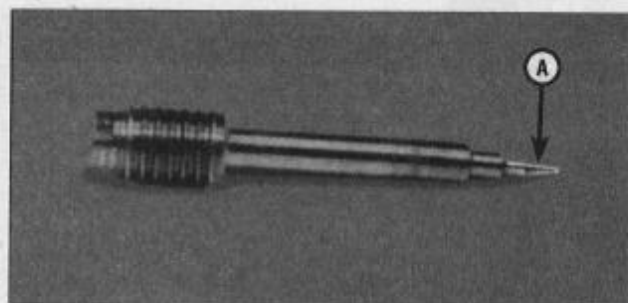
7.17 Check the tapered portion of the pilot screw (A) for wear or damage
