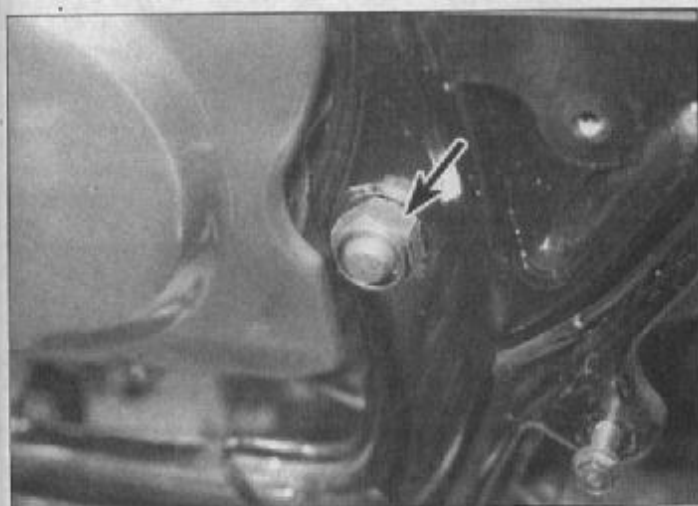
8.5 Remove the swingarm pivot shaft nut and withdraw the shaft
