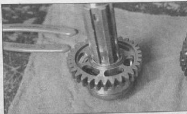
30.17b . . .and install second gear (flat side toward bearing), then secure it with a toothed washer and snap-ring
