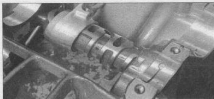
31.5a ...and slide the shift drum out of the fork and case
