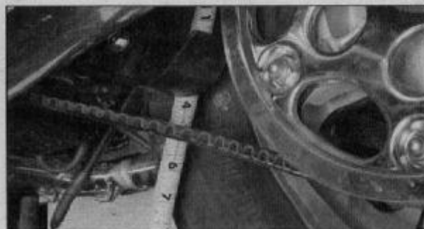
11.3 Push up on the bottom run of the belt and measure how far it deflects - if it's not within the specified limits, adjust the slack in the belt
