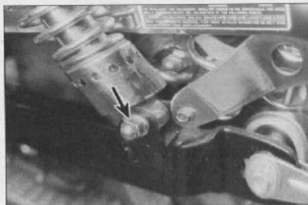
6.3c Remove the nut and bolt (arrow) from the lower end and remove the shock absorber
