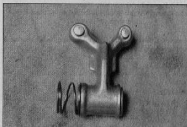
9.31 Remove the rocker arms and springs
