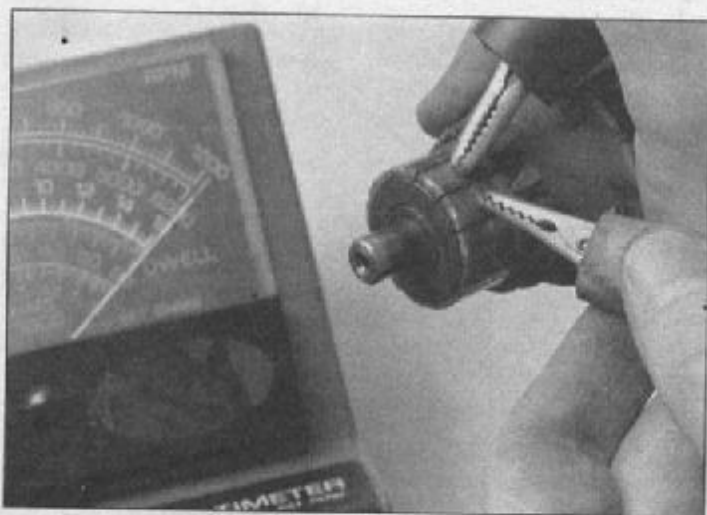
27.8a Continuity should exist between the commutator bars
