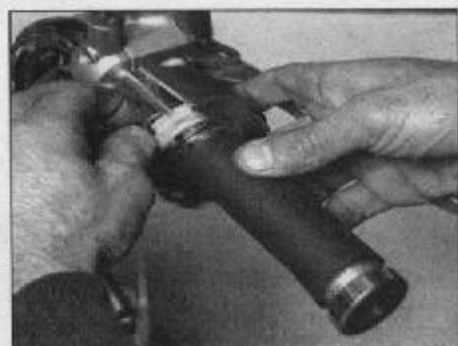
9.5a Lift the inner decelerator cable out of its groove, align it with the slots in the throttle pulley and slip the cable end out of the pulley ...
