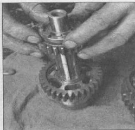
30.15k . . .and slide sixth gear off the shaft
