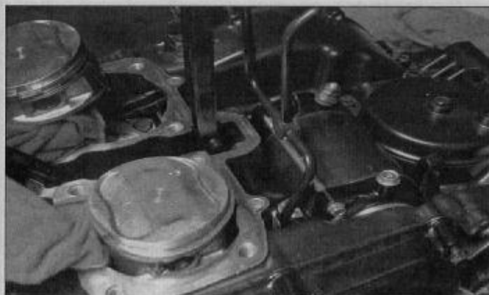
13.4 Lift the rear cam chain guide out of the engine (cylinder block removed for clarity)
