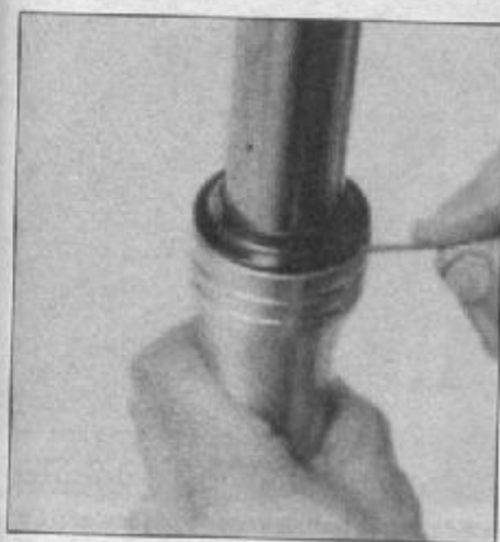
4.6 Pry the dust seal out of the outer tube with a small screwdriver
