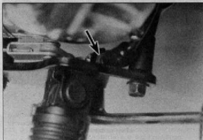
6.6 To adjust the rear brake light switch, hold the switch body and turn the locknut (arrow)
