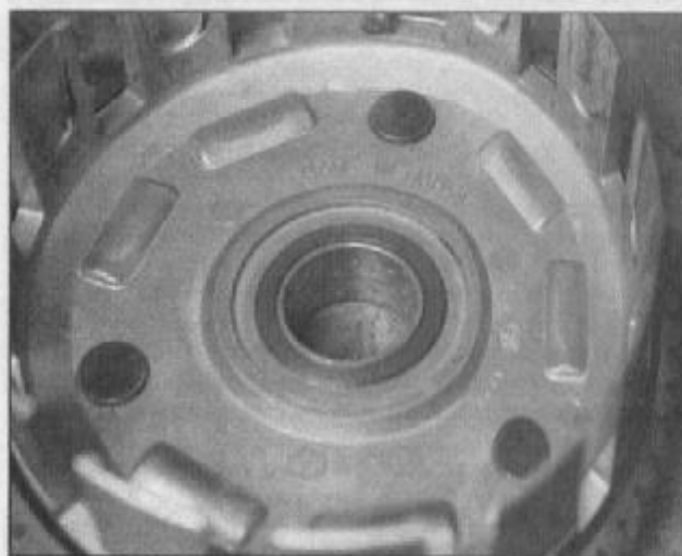
25.8 Inspect the bearing in the center of the clutch housing - replace the clutch housing if it's worn or damaged
