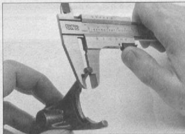
31.7 Measure the thickness of the shift fork ears
