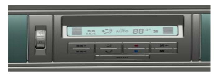
This control unit is connected to the front air conditioning control unit (master) via the CAN bus. It has the sole function of regulating control of the air conditioning system for the rear (3rd zone).
