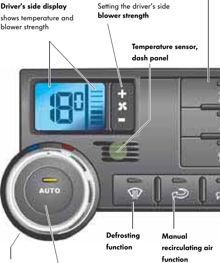
Auto button Automatic climate regulation driver's side The system independently regulates the climate zones that are set to Automatic according to the set temperature.
