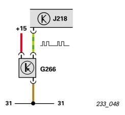
G266Sender for oil level/temperature J218Control unit for display unit in dash panel insert
