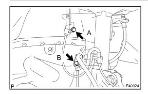
(b) Install the sensor harness clamp with the 2 bolts "A" and "B" to the body and shock absorber.
