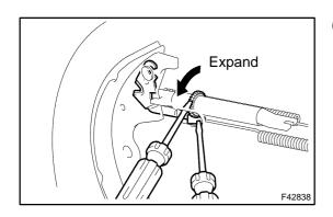
(b) Remove the hole plug, and turn the adjuster and expand the shoe until the drum locks.
