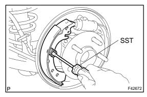
(b) Using SST, remove the cup, shoe hold–down spring and pin.
