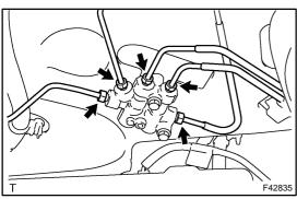
(b) Using SST, connect the 5 brake tubes to the proportioning valve assy.
