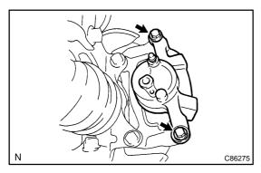
(b) Hold the cylinder slide pin and remove the 2 bolts.
