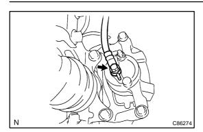
(b) Install a new gasket and flexible hose with the union bolt.
