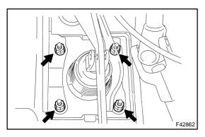
(c) Remove the 4 nuts and brake pedal support assy.
