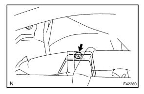
(c) Install the bolt to the brake pedal support sub–assy.
