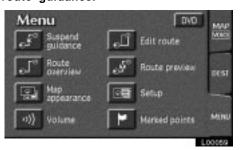
1. Touch the "MENU" tab on the screen to display the "Menu" screen and touch the "Route overview" switch.
