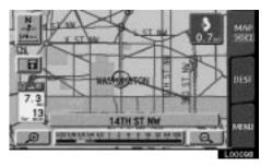
Touch or to change the scale of the map display. The scale bar and indicator at the bottom of the screen indicates the map scale menu. The scale runs from 1/32nd of a mile to 128 miles. Touch or until the scale bar changes normally. If you continue to touch on the switch, the scale bar
