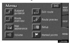
Touch the "MENU" tab on the screen to display the "Menu" screen. Then touch the "Volume" switch on the "Menu" screen.
