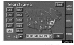
Touch one of the "US1" through "CAN" switches to select a search area. Touch the "OK" switch and the "Destination" screen returns.
