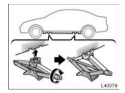
Position the jack at the correct jack point as shown. Rotate the load rest 90
