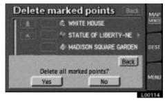
Either of the above messages appears depending on the type of deletion. If you want to delete, touch the "Yes" switch. To cancel the deletion, touch the "No" or "Back" switch.
