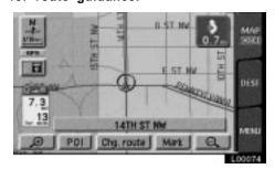
To display a particular type of point of interest on the screen, touch the "POI" switch on the map screen.
