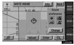
Touch the "Info." switch on the screen to display the selected destination name, address and telephone number.
