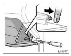
Open the glove box. Remove the screw with a Phillips-head screwdriver and slide the hook as shown.
