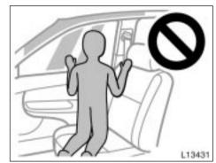
Do not allow a child to kneel on the passenger seat facing the passenger's side door. The side airbag and curtain shield airbag inflate with considerable speed and force; the child may be killed or seriously injured.
