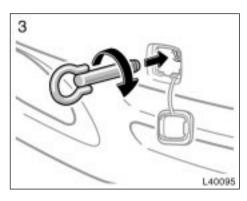
Secure the front towing eyelet to the hole on the bumper by turning clockwise.
