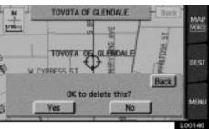
2. A selected point will appear. Also, a message will appear at the bottom of the screen. To delete, touch the "Yes" switch. To cancel the deletion, touch the "No" switch.
