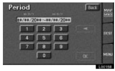
Touch the "Period" switch to display the "Memo list" as long as you desired. Touch numeral keys to input your desired search period. After inputting a search period, touch the "OK" switch. The "Memo list" screen will be displayed.
