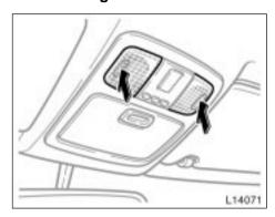
To turn on the front personal lights, push the lens. To turn the lights off, push the lens once again.
