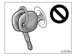
When starting the engine, do not use the key with other transponder keys around (including keys of other vehicles) and do not press other key plates against the key grip. Otherwise the engine may not start, or may stop soon after it starts. If this happens, remove the key once and then insert it again after taking off other transporter keys (including keys of other vehicles) from the ring or while gripping or covering them with your hand to start the engine.
