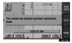
The above message appears and the fast distance calibration is automatically started. A few seconds later, the map screen returns.
