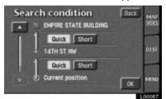
Touch the "Quick", "Short" or "Alternative" switch and touch the "OK" switch.
