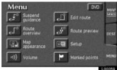
1. Touch the "MENU" tab on the screen to display the "Menu" screen and touch the "Marked points" switch.
