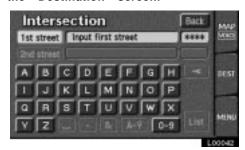
Input the name of the two intersecting streets which are located near the destination to be set.
