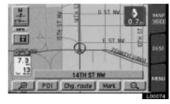
The current vehicle position mark appears in the center of the map screen. You can return to this map screen showing your current position at any time from any screen by touching the "MAP/VOICE" tab on the screen.
