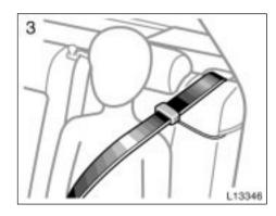
Buckle, position and release the seat belt. (For wearing the seat belt, see "—Front and rear seat belts" on page 42 in this section.) Make sure the shoulder belt crosses the shoulder.
