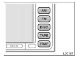
Push "AM", "FM", "DISC", "TAPE" or "TRAF" button to turn on the desired mode. The selected mode turns on immediately.
