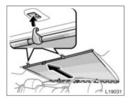
To raise the rear sunshade, pull the tab of the sunshade and hook it on the anchors. To lower the rear sunshade, pull the tab slightly to unhook the sunshade, and lower it slowly.
