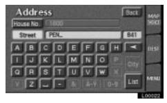
After each letter is input, the system searches the database for street names that match. Alphabet keys are dimmed if the database does not have a match for the next letter in the remaining list of matching street names.
