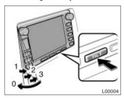
You can adjust the angle of the display by pushing the "TILT" button. Each push of the "TILT" button will tilt the display to position 1, 2, 3 and then back to 0 in that order.
