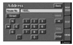
After inputting a house number, touch the "Enter" switch to display the screen which you can input a street name.
