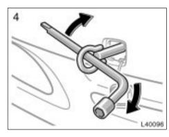
4. Tighten the front towing eyelet securely by a wheel nut wrench.
