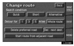
When you touch the "Chg. route" switch, the screen changes to a "Change route" screen that allows you to select the distance you want to detour. Touch one of the numeral keys to start the detour process. After detouring, the system returns to the original guidance route.
