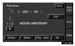
Touch the date you already input the memo. Displaying the memo you want to delete and then touch the "Delete" switch. A message appears on the display. To delete, touch the "Yes" switch. If not, touch the "No" switch.
