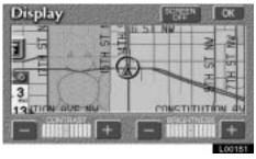
**BRIGHTNESS:** Adjusts the brightness of the screen.
