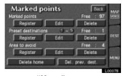
Touch the "Menu" tab on the screen to display the menu screen and touch the "Marked points" switch. Touch the "Del. prev. dest." switch.
