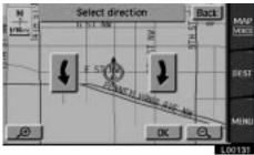
2. Touch either the left or right arrow to correct the direction of the current vehicle position mark.
