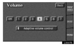
Touch any number to select the desired volume. Touching the "Off" switch turns the voice route guidance off. If you turn the "Adaptive volume control" on, the volume is turned up automatically when the vehicle speed exceeds 80 km/h (50 mph).
