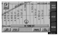
You can change the orientation of the map from the north-up to the heading up by touching the orientation symbol at the top left of the screen.
