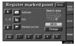
A screen similar to that for destination input appears. Input the address of the marked point in the same way as any destination input. See pages 10 through 24.
