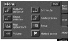
1. Touch the "MENU" tab on the screen to display the "Menu" screen and touch the "Map appearance" switch.
