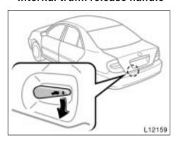
If a person is locked in the trunk, pull down the phosphorescent handle (illuminated for a while) on the inside of trunk lid in case of emergency to open the trunk lid.
