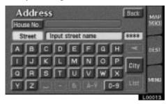
To type in an address etc., directly touch alphabet keys on the screen. If you touch a wrong letter, delete it using the switch. Touching the switch erases one letter.
