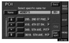
If you input the name of a specific point of interest and there are more than two sites with the same name, the "Dist Sort" switch will be shown. Touch the "Dist Sort" switch on the screen to display a listing of all items based on the distance from your current location.
