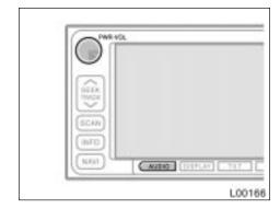
(a) Turning the system on and off POWER-VOL: Push this knob to turn the audio system on and off. Turn this knob to adjust the volume. The system turns on in the last mode used.
