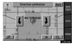
Touch the direction switches and adjust the direction. Touch the "OK" switch. The buzzer sounds when your vehicle approaches this icon in the direction that you set.
