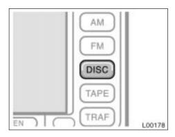
Push the "DISC" button if a compact disc is already loaded in the slot.
