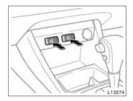
To turn on the seat heater, push the switch. To turn off the seat heater, push the switch once again.
