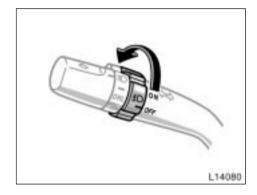
To turn on the front fog lights, twist the band of the headlight and turn signal switch lever. They will come on only when the headlights are on low beam.
