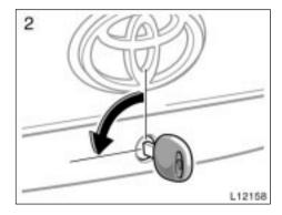
Close the trunk lid. Insert the master key and turn it counterclockwise to deactivate the trunk lid lock release lever.
