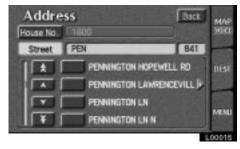
When a list is displayed, you can scroll or page through the list by using the appropriate switch.
