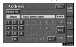
Touching the "A-Z" switch changes the screen back to the previous name input display.
