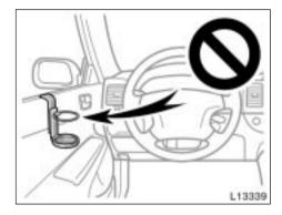
Do not attach a cup holder or any other device or object on or around the door. When the side airbag inflates, the cup holder or any other device or object will be hurled with great force or the side airbag may not activate correctly, resulting in death or serious injury. Likewise, the driver and front passenger should not hold things in their arms or on their knees.
