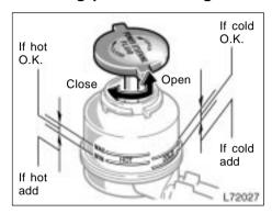
Check the fluid level through the reservoir. If necessary, add automatic transmission fluid DEXRON III.
