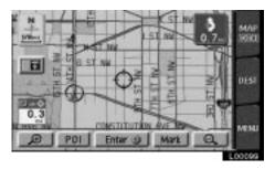
If you wish to look at a different point on the map other than your current vehicle position, you can bring the desired point to the center of the screen by using the scroll feature.
