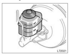
To check the fluid level, simply look at the see-through reservoir. The level should be between the "MAX" and "MIN" lines on the reservoir.
