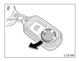
2. Remove the discharged transmitter battery.
