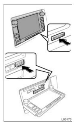
To stop and eject the cassette tape, push the "OPEN" button to lower the display. Push the "TAPE
