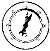
POOR VALVE SEATING AT IDLE
