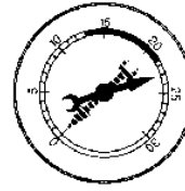
WORN RINGS OR DILUTED OIL RAPID ACCELERATION/ DECELERATION
