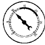
LATE VALVE TIMING, VACUUM LEAK AT IDLE
