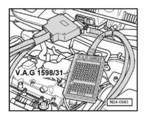
Connect test box V.A.G 1598/31 to control module wiring harness. The engine control module remains disconnected.
