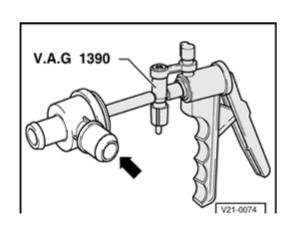
Operate vent valve on hand vacuum pump.
