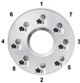
8-lug nut torque sequence
