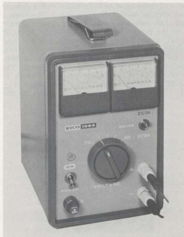
Fig. 4. Typical, filtered, DC power supply.
