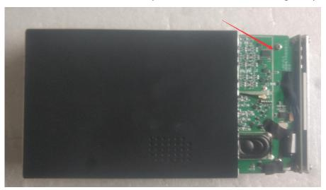
**Step 10:** Install the four screws of the shell.
