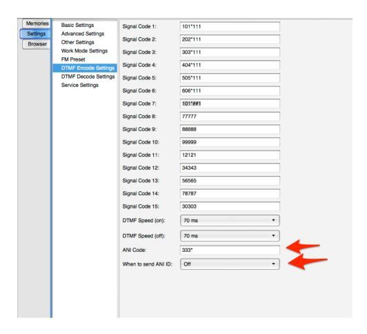
Now that we have enabled S-CODE to be transmitted at the end of transmission (via Menu 19); we can now select the S-CODE we want to transmit. We will do this from the Menu 17 (S-CODE).
