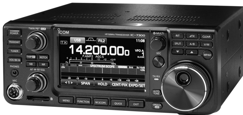
Fig 10 — The Icom IC-7300 is the first fully-SDR transceiver in a conventional HF transceiver package. Instead of a conventional superheterodyne conversion structure, digitization is performed directly at the RF signal frequency.
