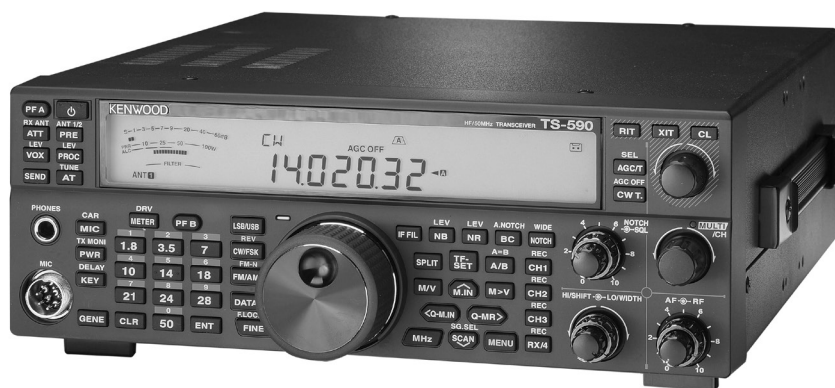
Fig 12 — The Kenwood TS-590SG offers a high performance receiver and many digital features.
