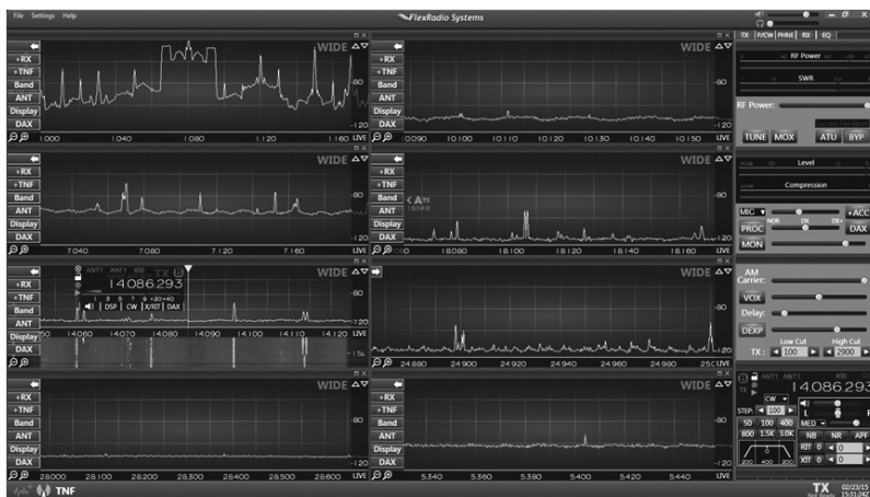
Fig 29 — One version of the main operating screen of SmartSDR for Windows operating software for the Flex 6000 series transceivers. In this case a FLEX-6700 has eight receivers and panadapters going simultaneously.
