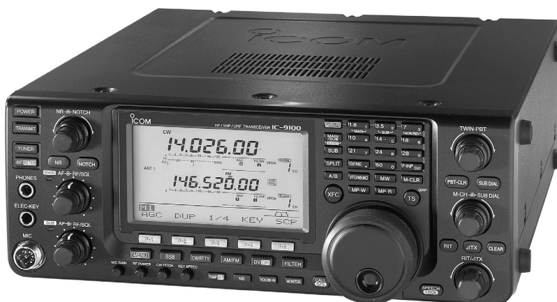
Fig 20 — The Icom IC-9100 transceiver offers coverage of 1.8 through 440 MHz with an option for 1.2 GHz operation.
