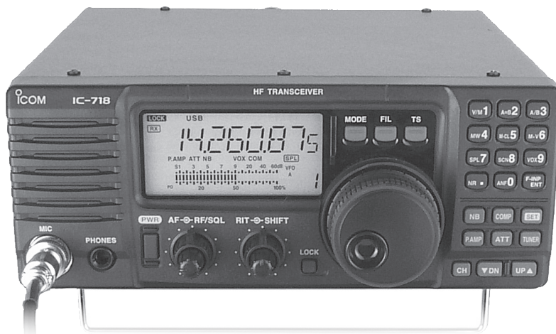
Fig 2 — The Icom IC-718 desktop HF transceiver.
