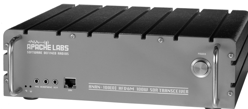
Fig 16 — The Apache Labs ANAN 100D HF and 6 meter DSP transceiver is the first of a new line of open-source software defined radios.
