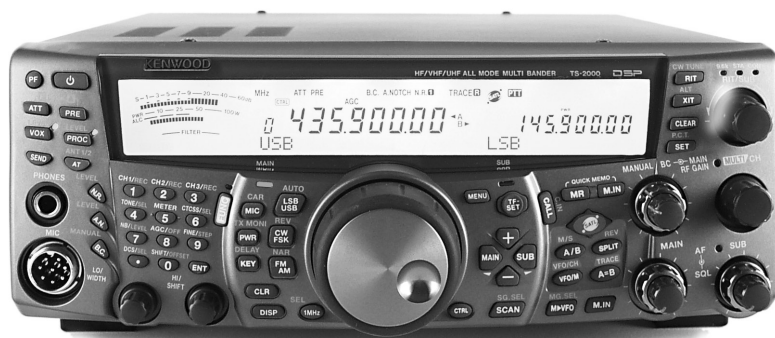
Fig 11 — Kenwood TS-2000. This transceiver operates on MF, HF, VHF, UHF, as well as the 1.2 GHz band with an option (TS-2000X version), providing broad frequency coverage in a single package.
