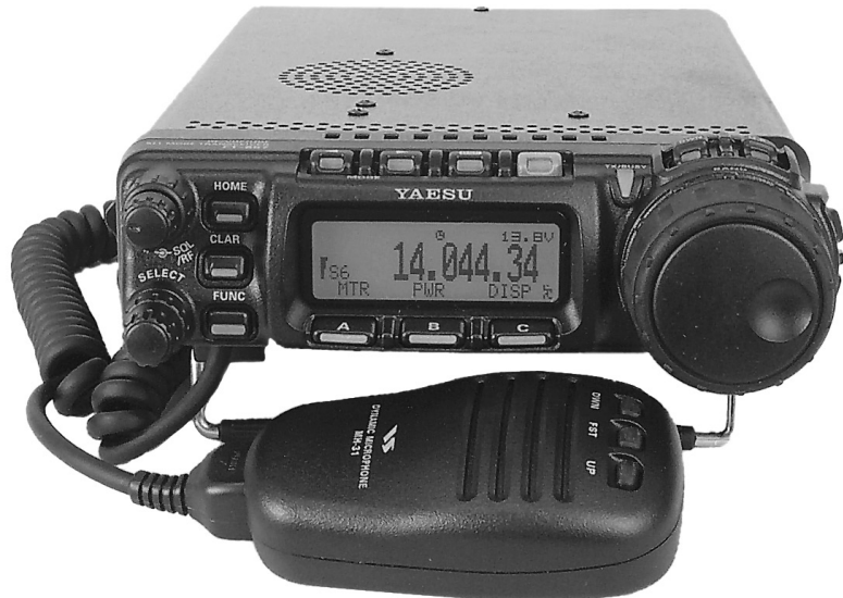
Fig 4 — The Yaesu FT-857D, an entry level transceiver with a mobile orientation and coverage up to 70 cm.
