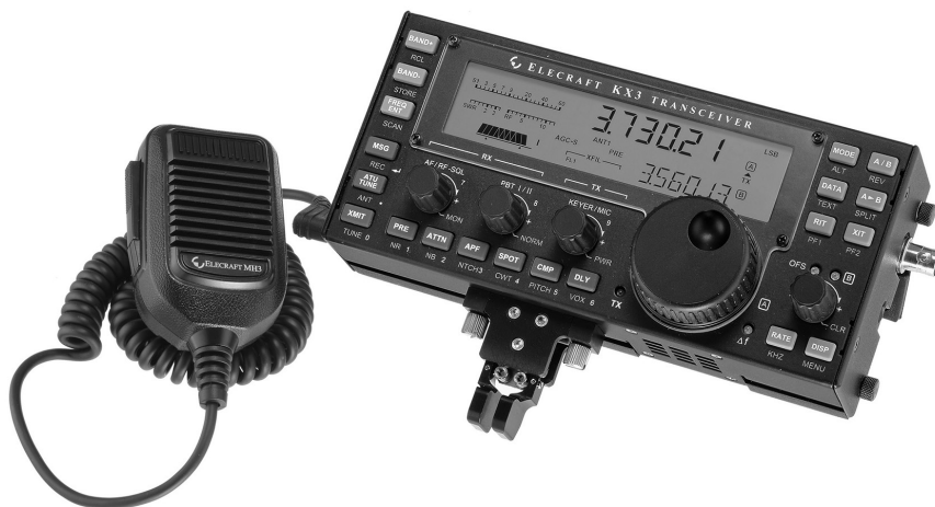
Fig 9 — The Elecraft KX3, when paired with the Elecraft KXPA100 100 W output HF and 6 meter linear amplifier can serve as flexible HF and VHF home station, as well as a easy to carry portable station.
