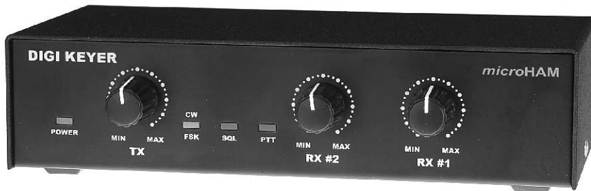
Fig 3 — The MicroHam Digi Keyer is an example of a multifunction sound card interface. Some commercial devices include CW keyers, transceiver control interfaces and support for multiple transceivers.
