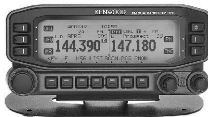
Fig 37 — The Kenwood TM-D710 is a dual-band FM transceiver with a built-in packet radio Terminal Node Controller (TNC) for digital communication.
