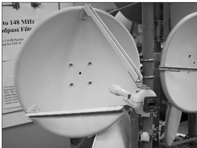
Fig 23 — As you can see, the feed source is directly in front, making this a center-fed dish.
