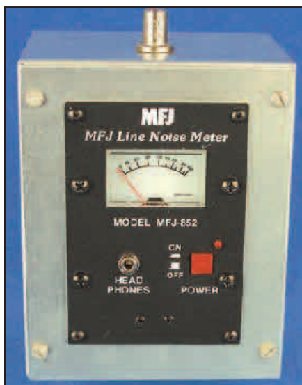
Figure 6 — Shielded MFJ-852 mounted in metal Bud box.
