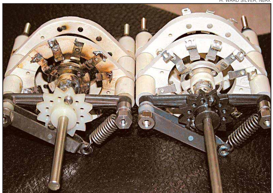
Figure 3—The band switch section on the left clearly shows the signs of destructive arcing.
