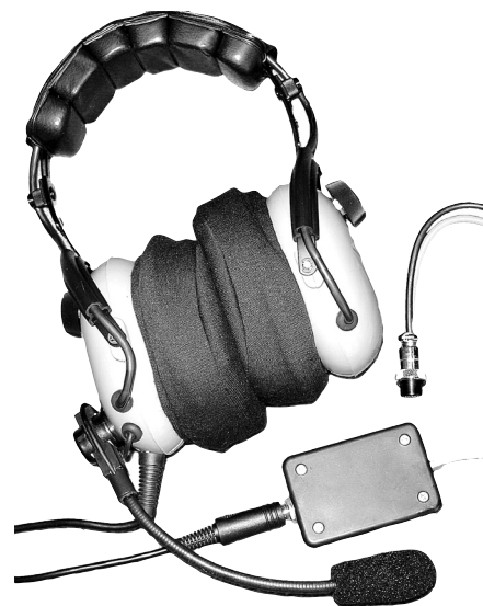
Fig 24.56 — A completed K0IZ headset/adapter. The black box contains the adapter circuit for the aviation headset.
