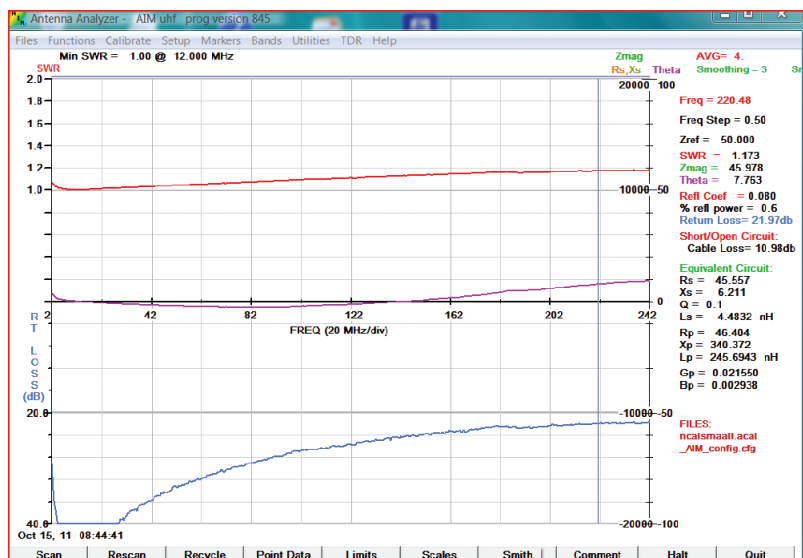
Figure 4 — AIMuhf data sweep of the bias T SWR with compensation.
