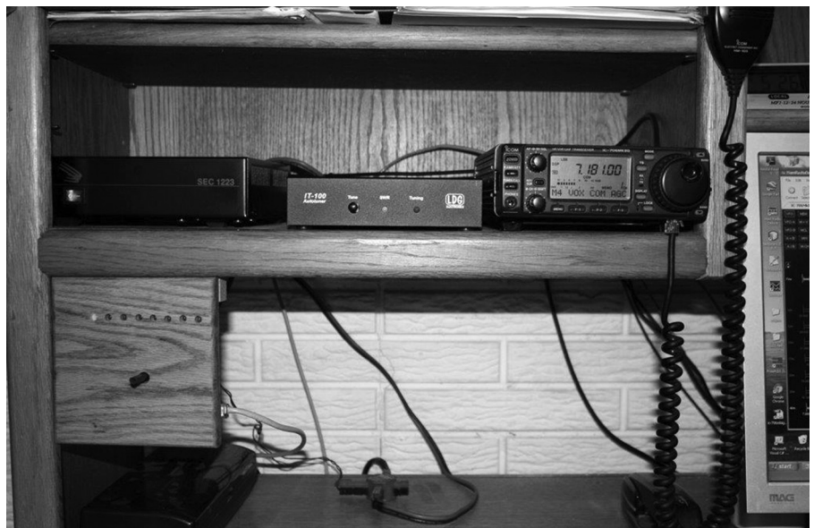
Figure 2 — This photo of my operating position shows my power supply, LDG Autotuner, and Icom IC-706 MKIIG radio. The antenna selector control panel is mounted behind a block of wood to match the operating position shelf. You can see the selector shaft, with the first of eight LEDs illuminated to show which antenna has been selected. I still have to add labels below the LEDs to help identify the antennas.
