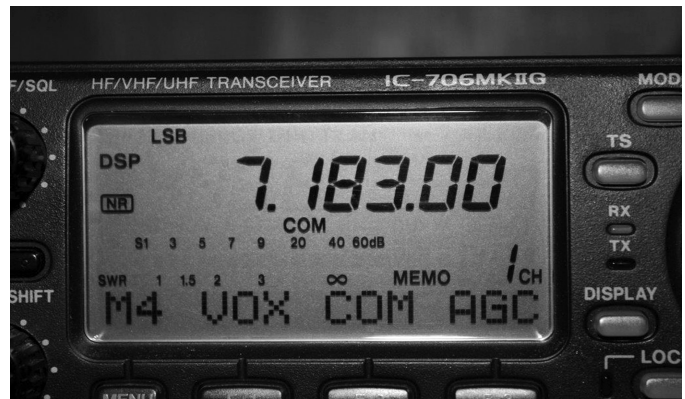
Figure 4 — In this close-up of the Icom radio display, there is no antenna connected. In this case, the S meter is showing no signal.
