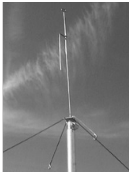
Fig 21.111 — K3MF's whip can be used to make a dual-band ground-plane antenna. Separate radials for 2 meters and 70-cm simplifies tuning. (Photo by K8CH)
