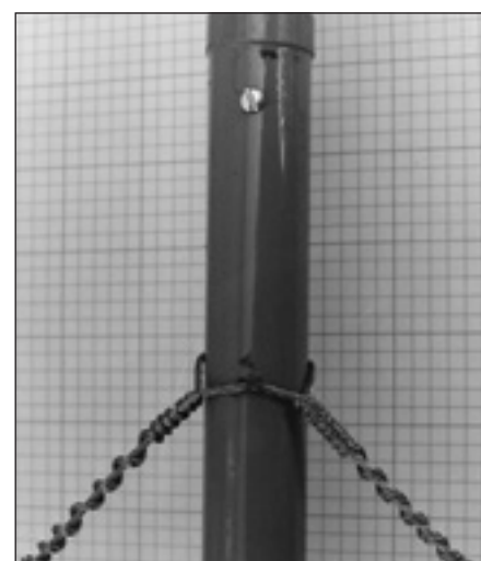
Fig 21.81 — Attaching quad wires to the spreaders must minimize stress on the wires for best reliability. This method (described in the text) cuts the chances of wind-induced wire breakage by distributing stress.
