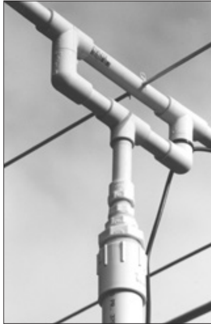
Fig 21.120 — The parasitic element mounting system, showing the placement of the hitch-pin clips and the shape of the clips.
