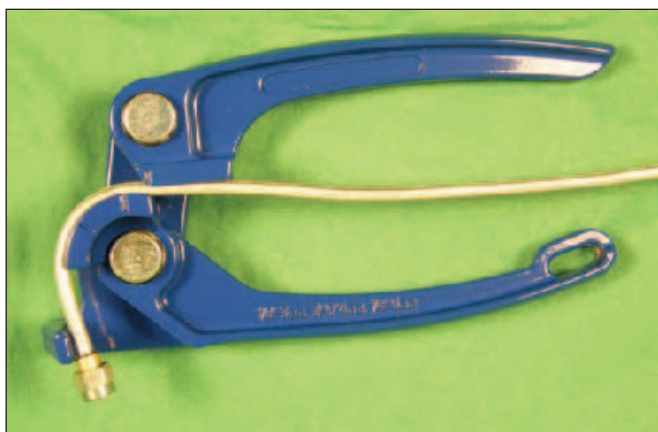
Figure 6 — Bending semirigid cable with a miniature tubing bender.
