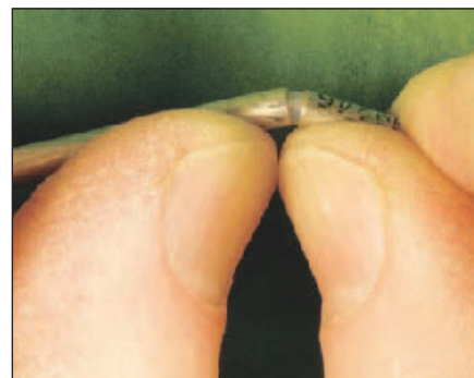
Figure 3 — Flex the cable with thumbs until the outer tubing snaps at the score line.
