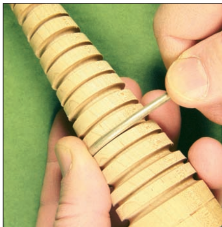
Figure 5 — Bending semirigid cable around a homemade bending jig.
