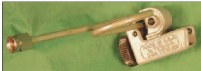
Figure 2 — Score the outer tubing with a miniature tubing cutter.
