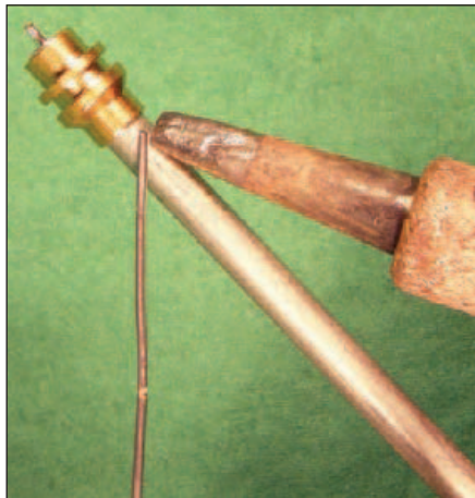
Figure 4 — Solder the connector body to the cable. Make sure to slide any necessary pieces on the cable first.
