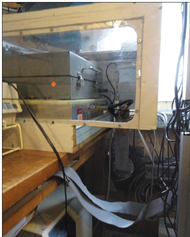
Figure 5 — The aluminum boxes contain the RF components for the A and B receivers.
