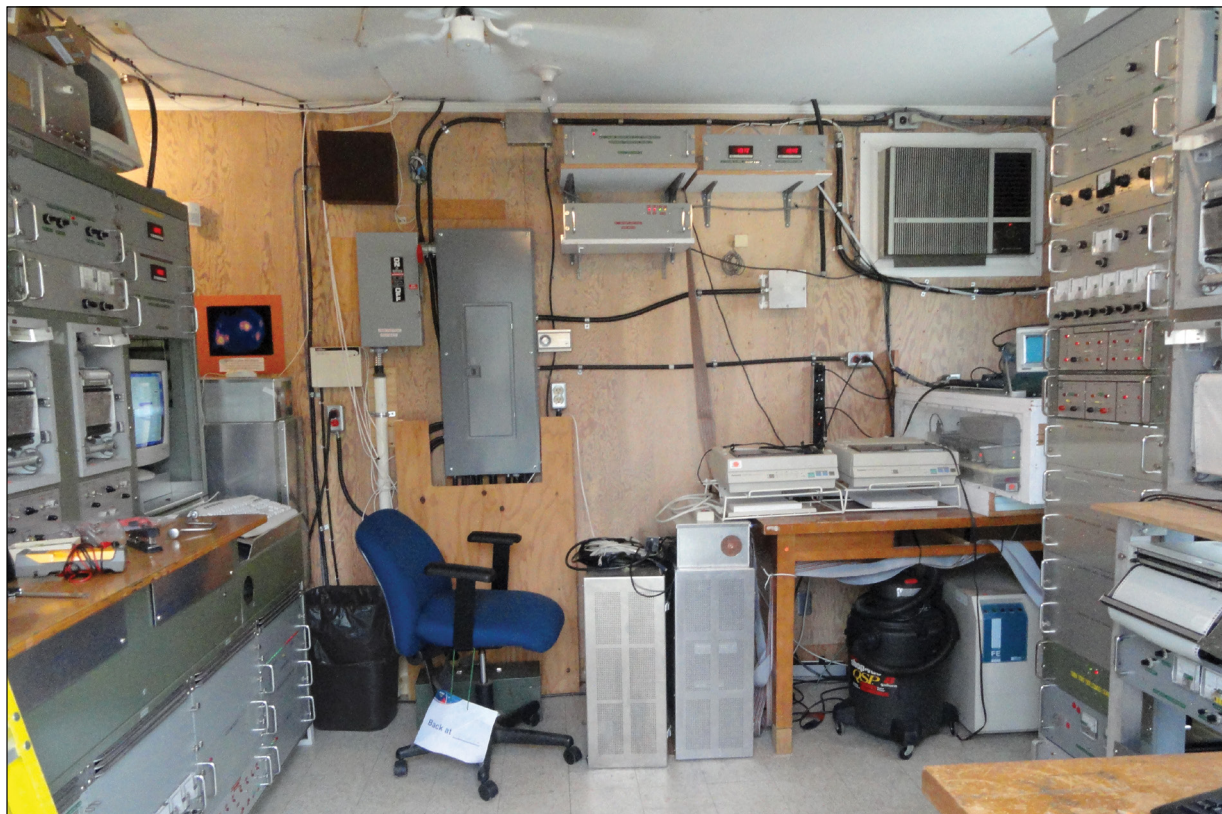
Figure 6 — A view in through the door of the solar hut. The FM1 rack is on the left, and the FM2 rack is on the right.
