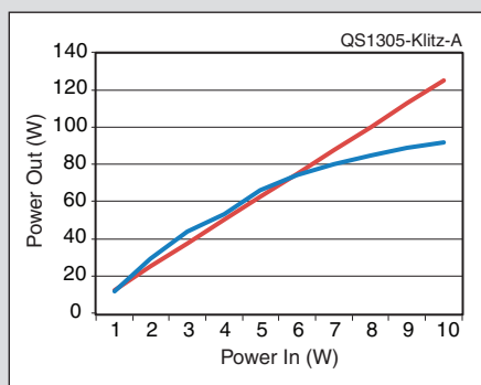
Figure A — Power output versus input, as measured in the ARRL Lab. A straight line (red) is shown for comparison.
