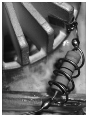
Figure 4 — Parasitic suppression chokes eliminate VHF oscillation by adding some resistance to the plate circuit at VHF. They consist of a few turns of wire over a resistor. The wire forms an inductor which passes signals at HF but forces VHF and higher-frequency signals through the resistor.
